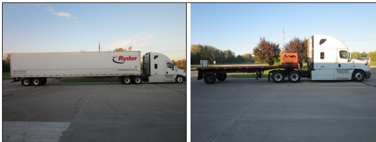
Figure 1. Class 8 Tractor with 53-Foot Dry Van Trailer and FMVSS No. 121 Unbraked Control Trailer
