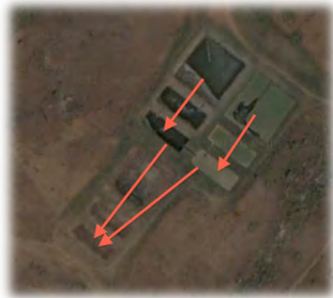
Figure 8: A view over Chancellor College WWTP. The process starts at the largest dark green pond, which is about 1600m 2 . By time of sampling only the last three ponds were working (Google Map Maker, 2012).
