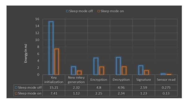
Figure 7.8: Comparison of energy consumption in sleep mode on and sleep mode off
