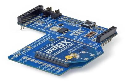
Figure 5.2: Arduino XBee Shield [4]
