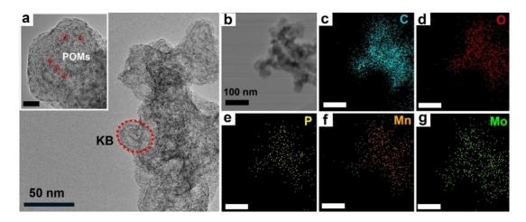
**Figure S9** (a) TEM images of **PMo<sub>12</sub>-MnL** loaded on KB (inset: HR-TEM images of **PMo<sub>12</sub>-MnL/KB**, scale bar: 5 nm). (b–g) Corresponding elemental mapping of C, O, P, Mn and Mo of **PMo<sub>12</sub>-MnL/KB**.
