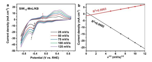
**Figure 17** (a) The CVs for SiW<sub>12</sub>-MnL/KB in 0.5 mol L<sup>-1</sup> N<sub>2</sub>-saturated KHCO<sub>3</sub> at different scan rate, (b) graph of peak current *vs.* square root of the scan rate.
