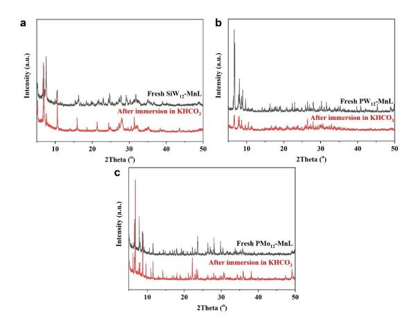
Figure S7. XRD patterns of the POMs-MnL after soaking in 0.5 M KHCO<sub>3</sub> solution.
