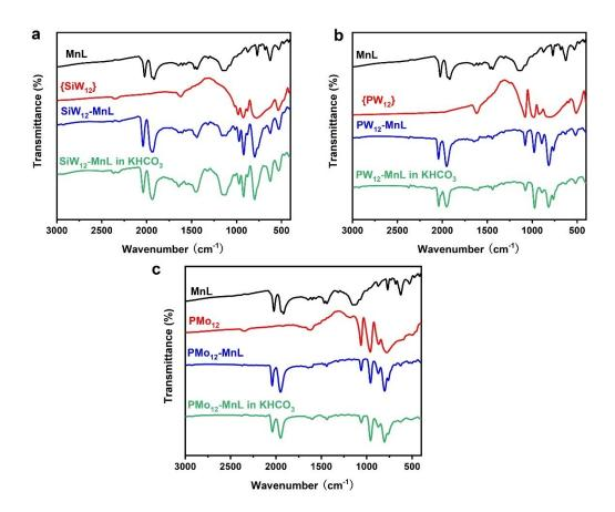
Figure S6. IR spectra of the POMs-MnL after soaking in 0.5 M KHCO<sub>3</sub> solution.
