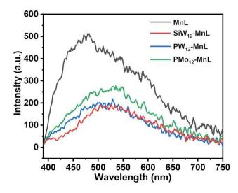
**Figure S29** the fluorescence diagram of MnL and POM-MnL ( $\lambda_{ex}$ = 380 nm)
