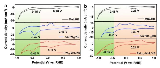
Figure S16 The CVs for MnL/KB,  $CsPW_{12}/KB$  and  $PW_{12}$ -MnL/KB (a) and for MnL/KB,  $CsPMo_{12}/KB$  and  $PMo_{12}$ -MnL/KB (b) in 0.5 mol L<sup>-1</sup> N<sub>2</sub>-saturated KHCO<sub>3</sub> at 0.05 V s<sup>-1</sup> scan rate.
