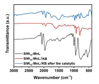
Figure S28 IR spectra of SiW<sub>12</sub>-MnL, SiW<sub>12</sub>-MnL/KB and SiW<sub>12</sub>-MnL/KB after catalytic reactions.
