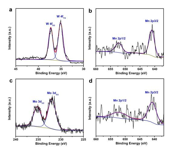
Figure S12 the XPS spectra of PW<sub>12</sub>-MnL/KB: (a) W, (b) Mn; the XPS spectra of PMo<sub>12</sub>-MnL/KB: (c) Mo, (d) Mn.
