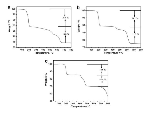
Figure S5 TG curves of SiW<sub>12</sub>-MnL (a), PW<sub>12</sub>-MnL (b) and PMo<sub>12</sub>-MnL (c).
