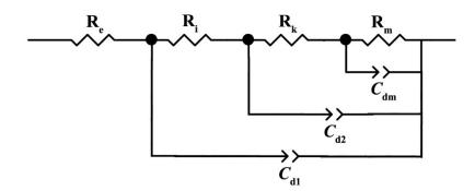
Figure S25 The equivalent circuit model.
