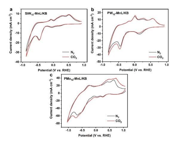
Figure 20 The CV curves of SiW<sub>12</sub>-MnL/KB (a),  $PW_{12}$ -MnL/KB (b) and  $PMo_{12}$ -MnL/KB (c) in 0.5 M N<sub>2</sub>-(black curve) or CO<sub>2</sub>- (red curve) saturated KHCO<sub>3</sub> electrolyte.
