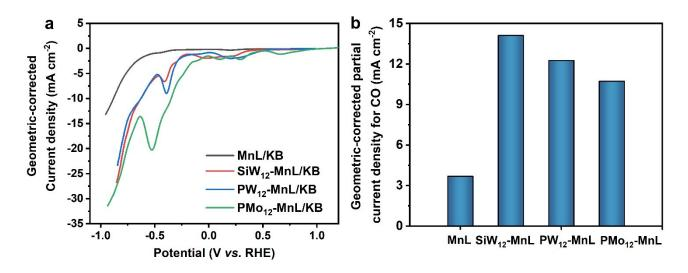
**Figure S21** (a) The geometric-corrected current density for MnL/KB and POMs-MnL/KB in 0.5 mol L<sup>-1</sup> CO<sub>2</sub>-saturated KHCO<sub>3</sub>, (b) The geometric area-corrected current densities for CO of POM-MnL/KB and MnL/KB.
