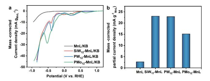
**Figure S24** (a) The mass activity (current per catalyst mass)-corrected current density for MnL/KB and POMs-MnL/KB in 0.5 mol L<sup>-1</sup> CO<sub>2</sub>-saturated KHCO<sub>3</sub>, (b) The mass activity (current per catalyst mass)-corrected current densities for CO of POM-MnL/KB and MnL/KB.
