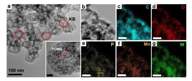
Figure S8 (a) TEM images of PW<sub>12</sub>-MnL loaded on KB (inset: HR-TEM images of PW<sub>12</sub>-MnL/KB, scale bar: 5 nm). (b–g) Corresponding elemental mapping of C, O, P, Mn and W of PW<sub>12</sub>-MnL/KB.
