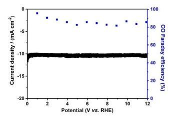
**Figure S26** Changes in current density and FE of SiW<sub>12</sub>-MnL loaded on KB over 12 h at - 0.72 V ( $\eta = 0.61$ ).
