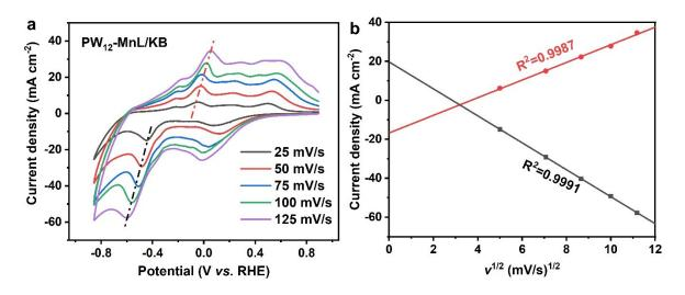
**Figure 18** (a) The CVs for  $PW_{12}$ -MnL/KB in 0.5 mol L<sup>-1</sup> N<sub>2</sub>-saturated KHCO<sub>3</sub> at different scan rate, (b) graph of peak current *vs*. square root of the scan rate.
