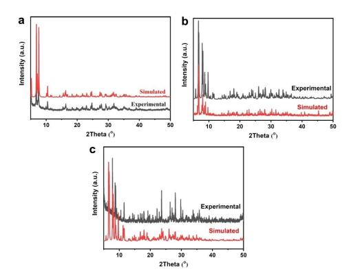
Figure S4 The powder X-ray diffraction patterns of  $SiW_{12}$ -MnL (a),  $PW_{12}$ -MnL (b) and  $PMo_{12}$ -MnL (c). Powder X-ray diffraction (PXRD, Figure S4) certified the structural integrity and phase purity of the crystalline POM-MnL composite catalysts, the experimental data are consistent with the simulated data are corresponded, which indicates that POM-MnL has been successfully prepared.
