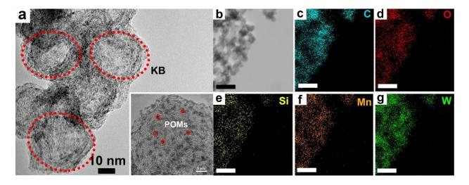
**Figure S27** (a) TEM images of  $SiW_{12}$ -MnL/KB after the catalytic reactions (inset: HR-TEM images of  $SiW_{12}$ -MnL after the catalytic). (b–g) Corresponding elemental mapping of C, O, Si, Mn and W of  $SiW_{12}$ -MnL/KB after the catalytic reactions.
