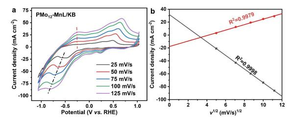
**Figure 19** (a) The CVs for  $PMo_{12}$ -MnL/KB in 0.5 mol L<sup>-1</sup> N<sub>2</sub>-saturated KHCO<sub>3</sub> at different scan rate, (b) graph of peak current *vs*. square root of the scan rate.
