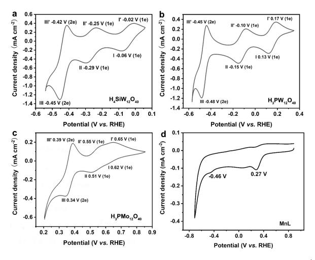
Figure S15 The CV curves of  $H_4SiW_{12}O_{40}(a)$ ,  $H_3PW_{12}O_{40}(b)$ ,  $H_3PMo_{12}O_{40}(c)$  in 0.5 mol L<sup>-1</sup>  $H_2SO_4$  solution (pH 0.3) and MnL in 0.5 mol L<sup>-1</sup> KHCO<sub>3</sub> (pH 8.2) solution at 0.05 V s<sup>-1</sup> scan rate.
