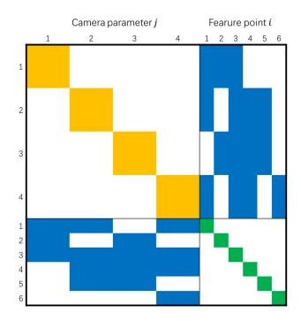
Figure 3.3: Hessian matrix demonstration of a small bundle adjustment problem (same as in Figure 3.2). The yellow block in  $\boldsymbol{B}$  is of size of  $9 \times 9$ ; the green block in  $\boldsymbol{C}$  is of size of  $3 \times 3$ ; the blue block in  $\boldsymbol{E}^T$  is of size of  $3 \times 9$ . If the blue blocks in  $\boldsymbol{E}^T$  is labeled with index (i, j), (i, j)-block is a non-zero matrix, if and only if when  $(i, j) \in \mathcal{S}$ .
