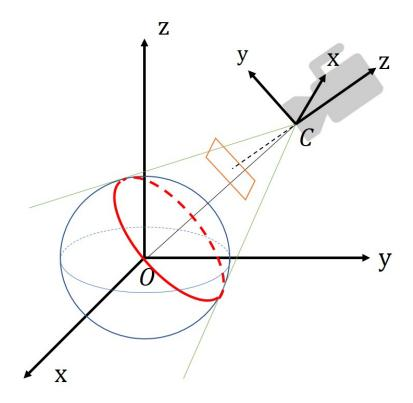
Figure 5.1: The structure of constructing a synthetic dataset. The orange parallelogram presents the image frames. The red circle defines a spherical cap, in which the feature points are visible for the current camera.
