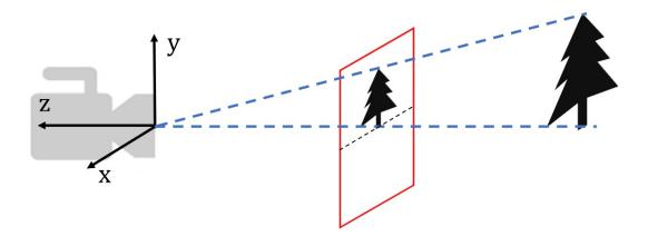
Figure 2.2: Perspective projection in a camera system. The red plane presents the projection plane located at (0, 0, -f). The real 3D object (tree) is proportional projected onto this plane.
