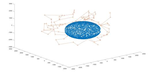
Figure 5.2: Synthetic dataset with 100 image frames and 5000 feature points in system O. The feature points are presented by blue "\*"; and the camera locations are presented as red " $\Delta$ ". All camera locations are connected together with red line according to its arranged order.
