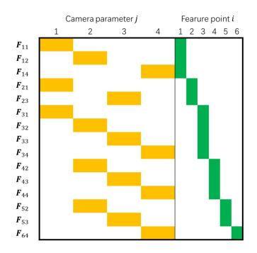
Figure 3.2: Jacobian matrix demonstration of a small bundle adjustment problem. There are 4 image frames and 6 feature points. The observation field is  $(ij) \in \{(11), (12), (14), (21), (23), (31), (32), (33), (34), (42), (43), (44), (52), (53), (64)\}$ . The yellow block in camera corresponding Jacobian part is of size of  $2 \times 9$ ; the green block in feature point corresponding Jacobian part is of size of  $\bullet \times 3$ .
