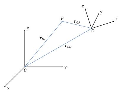
Figure 2.1: 3D coordinates (point P) transformation between coordinate system O and coordinate system C.
