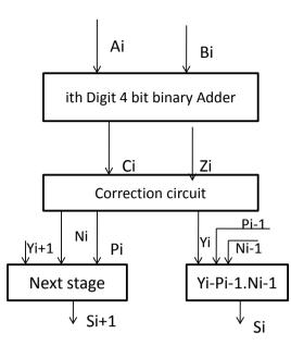
**Figure 9.** i<sup>th</sup> digit decimal adder.
