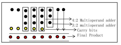
Figure 13. Addition of partial products using Multi Operand Adders.
