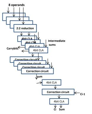
Figure 12. Multi operand adder with correction unit.
