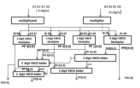
Figure 8. Four digit VBCD multiplier.
