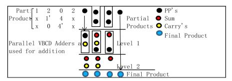
Figure 4. Addition of partial products using VBCD parallel adders.
