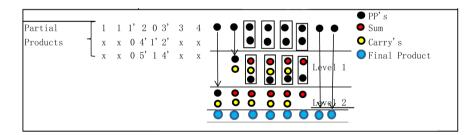
Figure 7. Addition of partial products using parallel adder.
