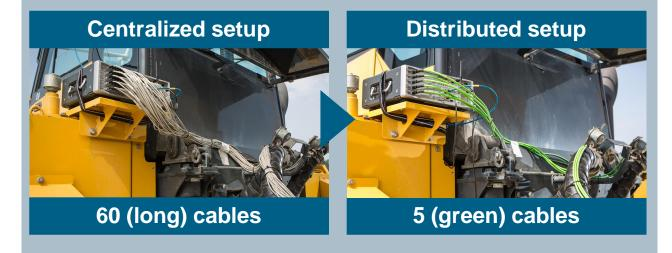
One single (green) cable carrying data and power for 12 channels simplifies instrumentation and repair
