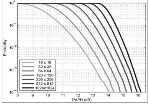
Fig. 4: Probability that the OFDM modulated 2D signal has a PAPR greater than a certain value for different image sizes
