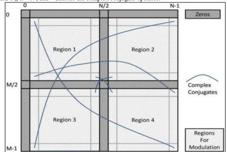
Fig. 3: Hermitian symmetric matrix used for DPSK-OFDM modulation. The IFFT of this matrix would have real-valued output on display. Bended lines show location of complex conjugate pairs
