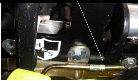
Bolt H&S bracket to coolant pipe bracket using supplied 5/16" bolt, washers, and nut. Tighten nut/bolt until snug, not tight.
