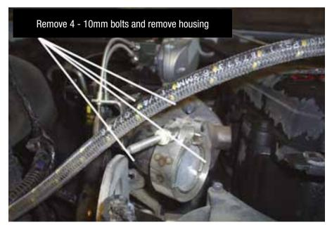
Remove 4 - 10mm bolts. If pick-up model install front block off plate with factory 15mm bolts. If cab & chassis model skip to next step.
