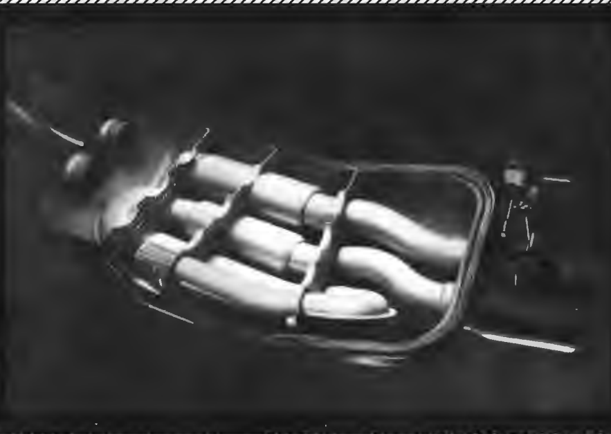
BMW 2.8-liter engine... Innovative switch-type muffler on the 328i as the optimum solution to the old conflict of interests between maximum power and efficient noise control.
