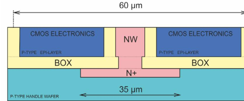
pixel block schematic
