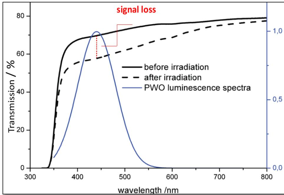
tested using  $\gamma$ -rays:  $\sim 1.2$  MeV
