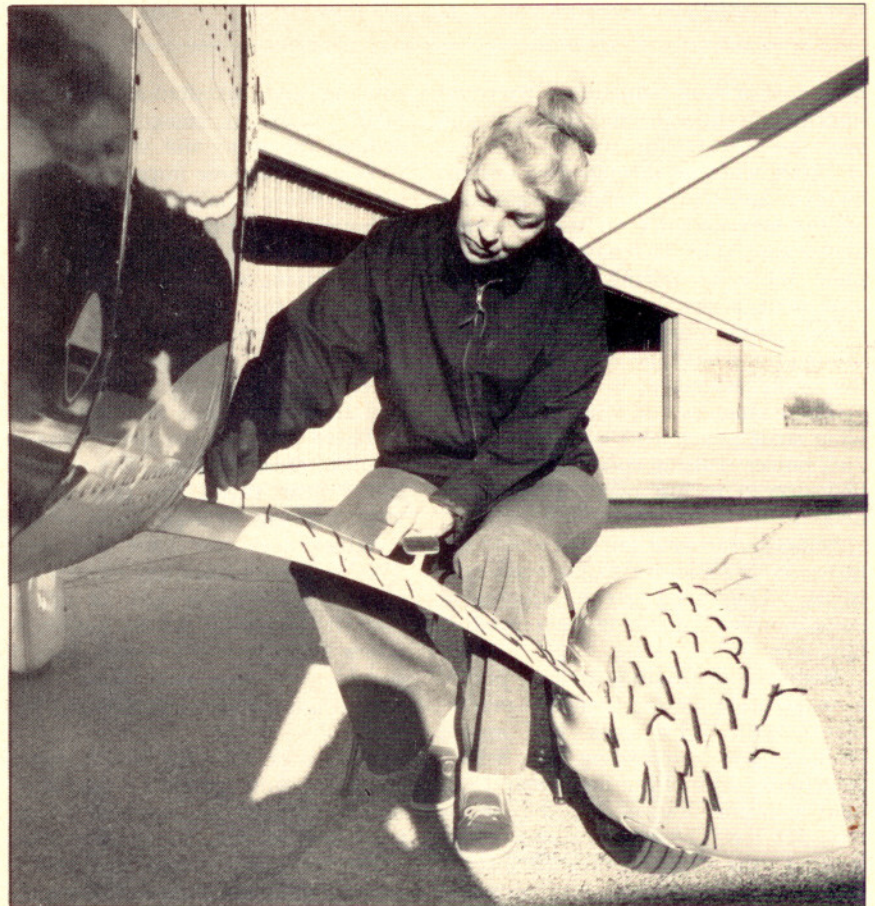
Extensive testing established drag characteristics of the aircraft. Julia applies tufts of yarn prior to a test of the main gear and wheel pants.
