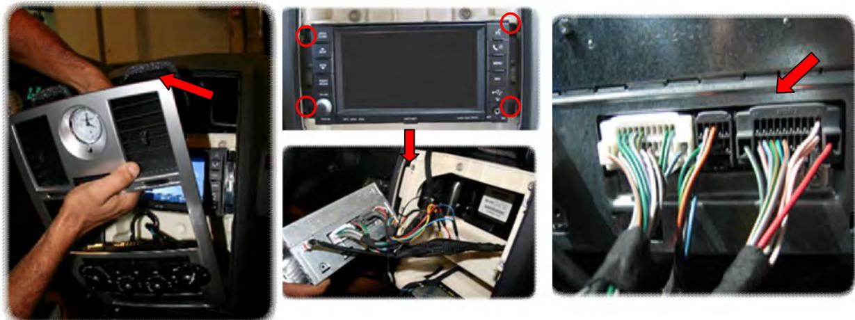
Unscrew the 4 torx and pull out the head unit. Disconnect the black 22-pin connector from the head unit. Cut the white/orange lead (pin 13) and the white lead (pin 2) of the black 22-pin connector and connect it according to the connection diagram on the page „connections“ to the cable connector of the IF-TF1280.
