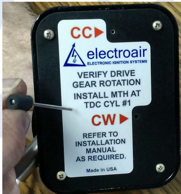
Figure 7: Installation of MTH Alignment Pin
