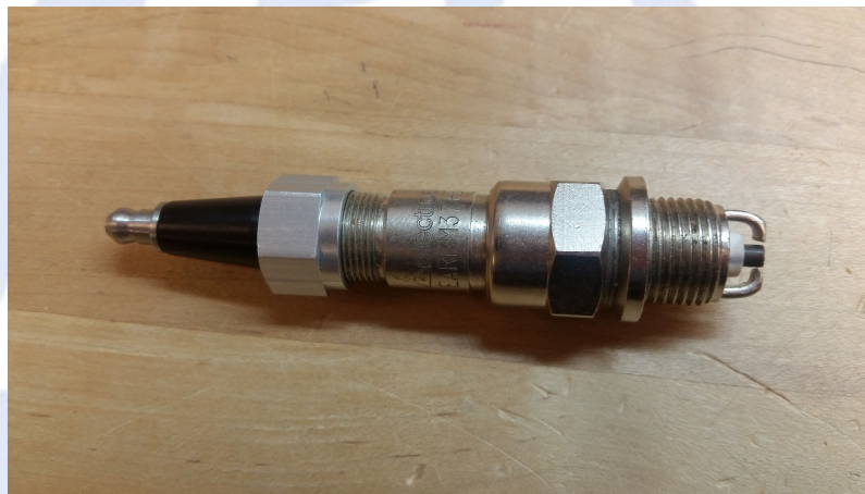
Figure 13: Spark Plug Tower Attached to Spark Plug
