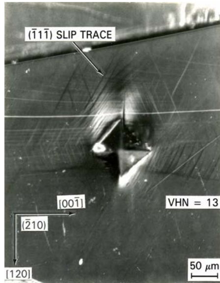
Fig. 32. Slip-initiated cracking at plane intersections in AP (ammonium perchlorate). 185
