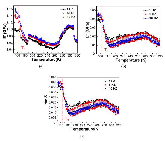
Figure 6. Temperature dependences of (a) storage modulus, E', (b) loss modulus, E'', and (c) loss factor  $tan\delta$  of  $[(CH_3)_2NH_2][Fe(HCOO)_3]$  single crystals at frequencies of 1–10 Hz determined by DMA during heating at the rate of 2 K/min. The vertical dash-dotted line indicates the ferroelectric transition temperature  $T_c \sim 164$  K.
