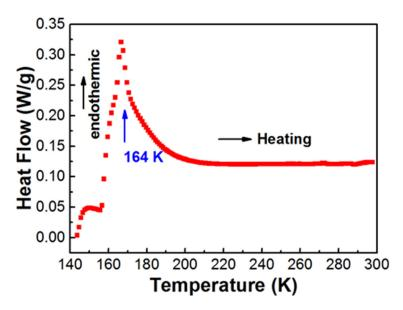
**Figure 3.** DSC curve of [(CH<sub>3</sub>)<sub>2</sub>NH<sub>2</sub>][Fe(HCOO)<sub>3</sub>] at the heating rate of 5 K/min.
