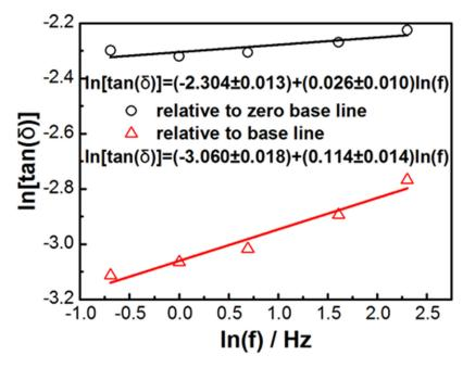
**Figure 9.** Double logarithmic plot ln(tan  $\delta$ ) vs. ln(f) for the peak height of tan  $\delta$  near 164 K for [(CH<sub>3</sub>)<sub>2</sub>NH<sub>2</sub>][Fe(HCOO)<sub>3</sub>] pellets fitting by power law tan  $\delta$  = Af<sup>n</sup>.
