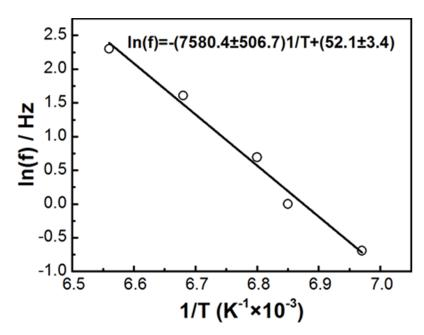
**Figure 8.**  $\ln(f)$  vs. 1/T for the peaks of temperature dependences of  $E''_T/E''_{298}$  near 145 K for  $[(CH_3)_2NH_2][Fe(HCOO)_3]$  pellets fitting by Arrhenius equation  $f = f_0 \exp(-E_a/RT)$ .
