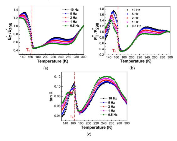
Figure 7. Temperature dependences of (a) the normalized storage modulus,  $E'_T/E'_{298}$ , (b) the normalized loss modulus,  $E''_T/E''_{298}$ , and (c) loss factor  $\tan \delta$  of [(CH<sub>3</sub>)<sub>2</sub>NH<sub>2</sub>][Fe(HCOO)<sub>3</sub>] pellets at frequencies of 0.5–10 Hz determined by DMA during heating at the rate of 2 K/min. The vertical dash-dotted line indicates the ferroelectric transition temperature  $T_c \sim 164$  K.
