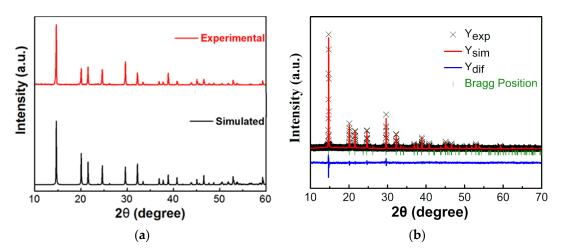
**Figure 1.** Powder XRD patterns of  $[(CH_3)_2NH_2][Fe(HCOO)_3]$  at room temperature, (**a**) the experimental and simulated XRD patterns, (**b**) Rietveld fit of XRD pattern. The simulated XRD pattern was for rhombohedral  $R_3$ c structure (CCDC 780885) [17].
