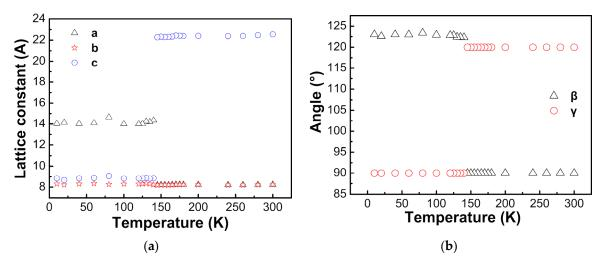
Figure 5. Temperature dependences of lattice parameters, (a) lattice constant, (b) angles.
