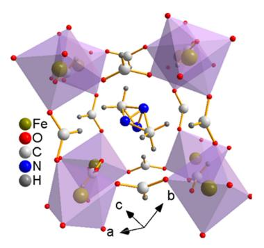
**Figure 2.** The rhombohedral R3c structure [17] of [(CH<sub>3</sub>)<sub>2</sub>NH<sub>2</sub>][Fe(HCOO)<sub>3</sub>] at room temperature. 3.2. *DSC*
