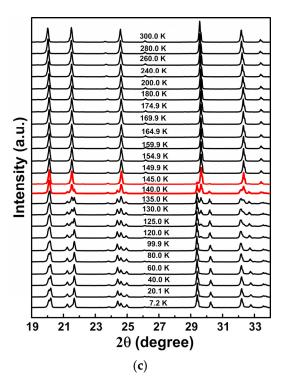
**Figure 4.** Powder XRD patterns of  $[(CH_3)_2NH_2][Fe(HCOO)_3]$  between 10 K and 300 K, with diffraction angle 20 in the range of (a)  $10-70^{\circ}$ , (b)  $14-15.5^{\circ}$ , (c)  $19-34^{\circ}$ .
