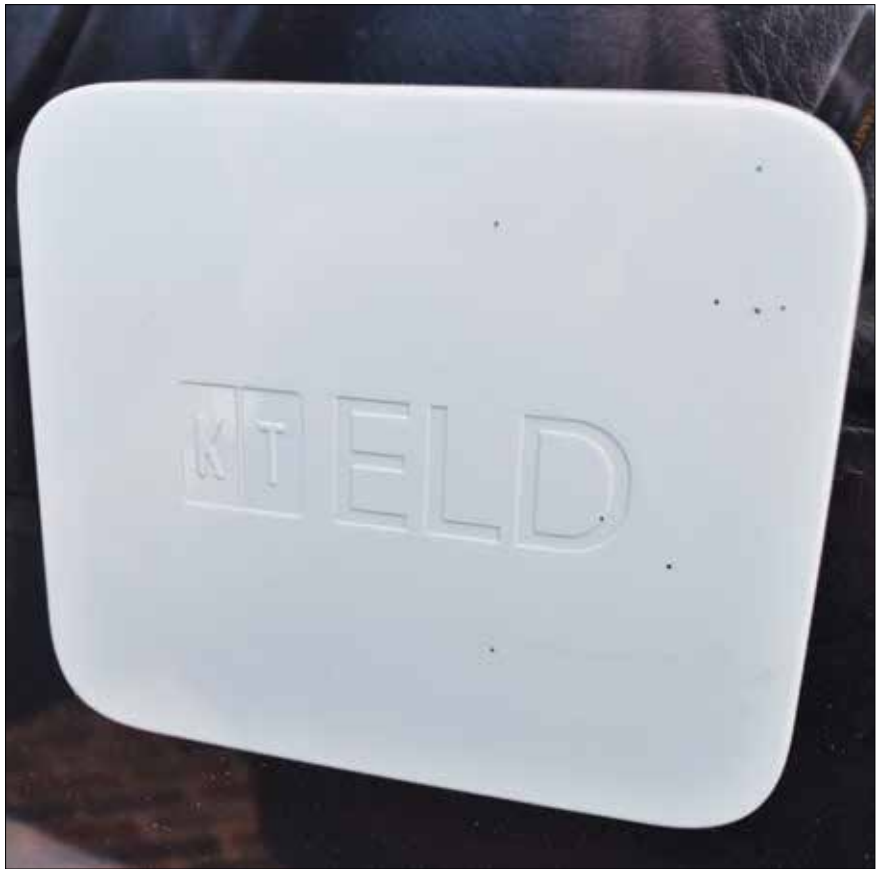
The KeepTruckin BYOD-style ELD "black box" connects to the ECM via cable and plugin. KeepTruckin recommends users mount the device in the dash to maintain a clear GPS connection. The device pairs with the KT app on a smartphone or tablet via Bluetooth connection, optionally via USB.
