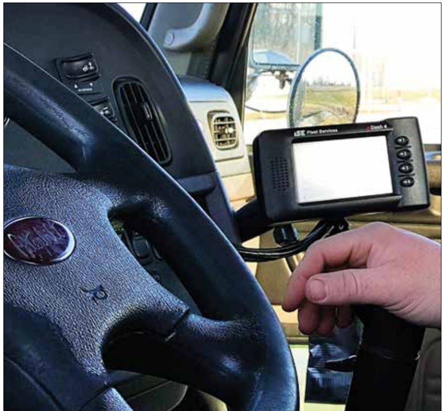
ISE Fleet Services' eFleetSuite baseline compliance device is a dedicated unit with its own cellular data connection but without a lot of extra functionality beyond logs.
