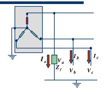
The terminal unbalance currents at the fault point can be transferred into their sequence components as follows:
