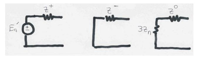
During a fault  $Z^+ \approx Z^- \approx X_d$ ". The zero sequence impedance is usually substantially smaller. The value of  $Z_n$  depends on whether the generator is grounded
