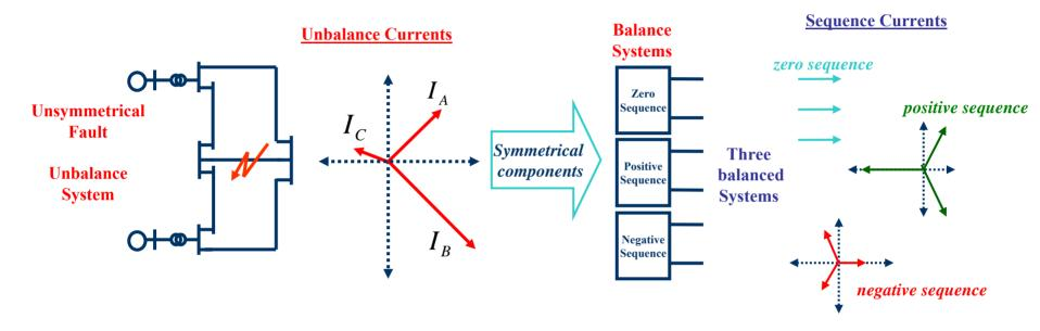
Assuming three unbalance voltage phasors,  $V_A$ ,  $V_B$  and  $V_C$  having a positive sequence (abc). Using symmetrical components it is possible to represent each
