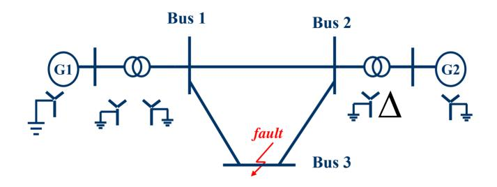
For the generators assume  $Z^+ = Z^- = j0.2$ ;  $Z^0 = j0.05$ For the transformers assume  $Z^+ = Z^- = j0.05$ For the lines assume  $Z^+ = Z^- = j0.1$ ;  $Z^0 = j0.3$ Assume unloaded pre-fault, with voltages =1.0 p.u.
