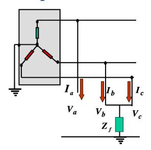
Note, because of the path to ground the zero sequence current is no longer zero.
