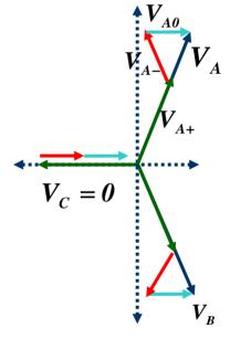
Synthesis Unsymmetrical phasors using symmetrical components
