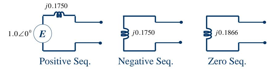
The fault type then determines how the networks are interconnected
