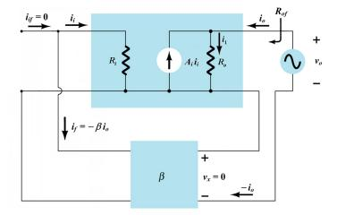
We can calculate the closed-loop output resistance (i.e., as a Thévenin equivalent resistance) by using the test voltage method as shown in the figure above. Note that as the feedback network is ideal, internal resistance of the feedback network is zero. So,  $v_x=0$  and  $v_o=i_1R_o+v_x=i_1R_o$ . Also as  $i_{if}=0$ ,  $i_i=-i_f=\beta i_o$ . Hence, output resistance  $R_{of}$
