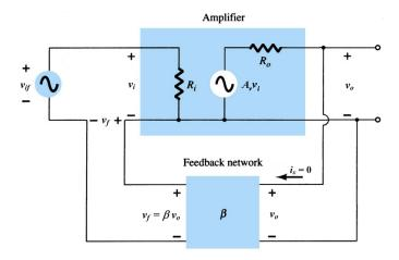
From the above figure, we can quickly derive the closed-loop no-load gain  $A_{\it vf}$  where
