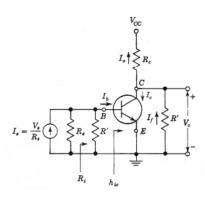
Now, the feedback gain  $\beta$  is given by  $\beta = \frac{i_f}{v_o} = \frac{i_f}{-i_f R'} = -\frac{1}{R'}$
