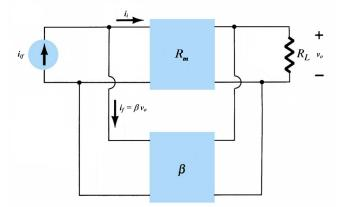
Voltage-shunt feedback amplifier is actually a closed-loop transresistance amplifier as shown below. We are going to find the derive the no-load gain  $R_{mf}$ , input resistance  $R_{if}$  and output resistance  $R_{of}$  of this closed-loop system.
