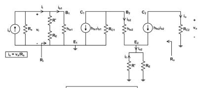
Now, the feedback gain eta is given by  $eta=rac{i_f}{i_o}=rac{R_E}{R'+R_E}$
