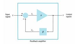
From the figure above we can calculate the closed-loop gain (i.e., gain with feedback),  $A_f=rac{Y}{X}$  as follows
