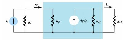
From the closed-loop amplifier diagram above, we can also find the overall closed-loop current gain  $A_{\mathit{Isf}}$ , as
