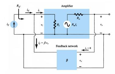
From the above figure, we can quickly derive the closed-loop input resistance  $R_{\it if}$
