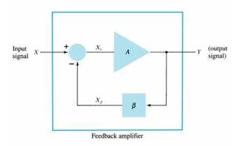
The effects of the negative feedback on an amplifier can be summarized as follows.
