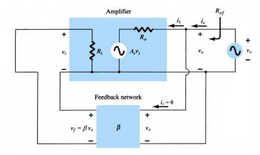
We can calculate the closed-loop output resistance (i.e., as a Thévenin equivalent resistance) by using the test voltage method as shown in the figure above. Note that as the feedback network is ideal, internal resistance of the feedback network is infinity. So,  $i_x=0$  and  $i_o=i_1+i_x=i_1$ . Also as  $v_{if}=0$ ,  $v_i=-v_f=-\beta v_o$ . Hence, output resistance  $R_{of}$
