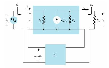
Let us derive no-load gain  $G_{m\!f}$  , input resistance  $R_{i\!f}$  and output resistance  $R_{o\!f}$  of the current-series feedback system in terms of the open-loop amplifier parameters  $G_m$ ,  $R_i$  and  $R_o$ .
