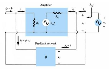
We can calculate the closed-loop output resistance (i.e., as a Thévenin equivalent resistance) by using the test voltage method as shown in the figure above. Note that as the feedback network is ideal, internal resistance of the feedback network is infinity. So,  $i_x=0$  and  $i_o=i_1+i_x=i_1$ . Also as  $i_{if}=0$ ,  $i_i=-i_f=-\beta v_o$ . Hence, output resistance  $R_{of}$
