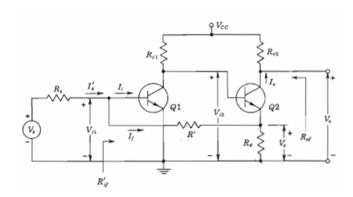
**Solution:** Output and input networks have two common elements R' and  $R_E$  which provide feedback in this circuit. It is connected in parallel (i.e., shunt connection) to the input circuitry. The feedback signal  $i_f$  is the voltage through resistor R'. Output signal sampled is output current  $i_{\mathcal{O}}$ . So, this circuit has **current-shunt feedback**.
