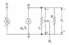
Now, the feedback gain eta is given by  $\left| \ eta = rac{v_f}{v_o} = 1
