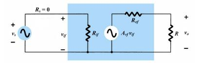
From the closed-loop amplifier diagram above, we can also find the overall closed-loop voltage gain  $A_{V\!sf}$ , as
