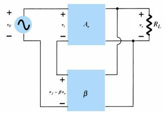
Voltage-series feedback amplifier is actually a closed-loop voltage-gain amplifier as shown below. We are going to find the derive the no-load gain  $A_{vf}$ , input resistance  $R_{if}$  and output resistance  $R_{of}$  of this closed-loop system.
