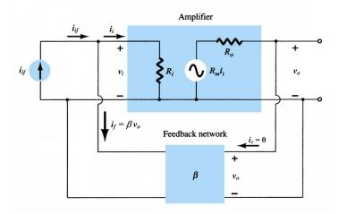
From the above figure, we can quickly derive the closed-loop no-load gain  $R_{m\!f}$  where
