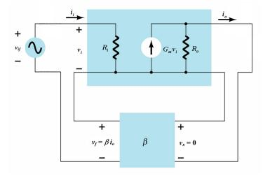
From the above figure, we can quickly derive the closed-loop no-load gain  $G_{\it mf}$  where
