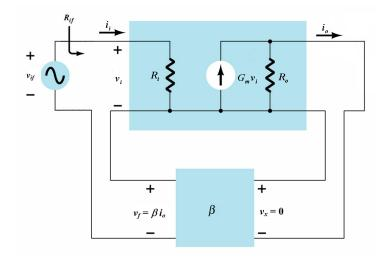
From the above figure, we can quickly derive the closed-loop input resistance  $R_{\it if}$
