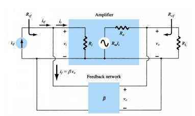
Let us derive no-load gain  $R_{mf}$ , input resistance  $R_{if}$  and output resistance  $R_{of}$  of the voltage-shunt feedback system in terms of the open-loop amplifier parameters  $R_m$ ,  $R_i$  and  $R_o$ .
