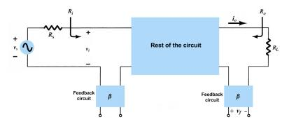
iv. Open-loop circuit diagram for current-shunt feedback
