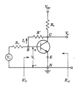
Solution: Output and input network have one common element R' which provides feedback in this circuit. It is connected in parallel (i.e., shunt connection) to the input circuitry. The feedback signal  $i_f$  is the current through resistor R'. Output signal sampled is output voltage  $v_o$ . So, this circuit has voltage-shunt feedback.
