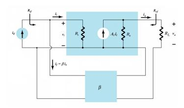
Let us derive no-load gain  $A_{i\!f}$  , input resistance  $R_{i\!f}$  and output resistance  $R_{o\!f}$  of the current-shunt feedback system in terms of the open-loop amplifier parameters  $A_i$ ,  $R_i$  and  $R_o$ .
