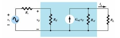
From the closed-loop amplifier diagram above, we can also find the overall closed-loop transconductance gain  $G_{M\!s\!f}$ , as
