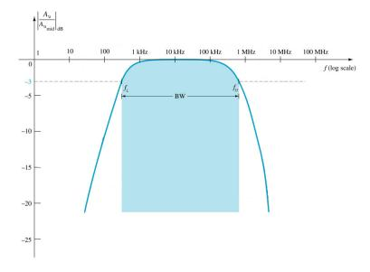
Bandwidth BW is the difference between the higher cut-off frequency  $f_H$  and the lower cut-off frequency  $f_L$  of the amplifier, i.e.,
