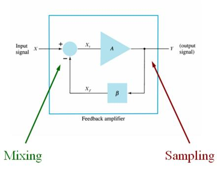
The output signal is **sampled** and fed back to the system and **mixed** with the input signal. Here, we are going to analyze the possible sampling and mixing types.
