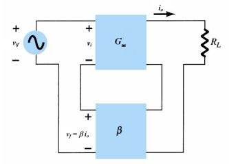
Current-series feedback amplifier is actually a closed-loop transconductance amplifier as shown below. We are going to find the derive the no-load gain  $G_{mf}$ , input resistance  $R_{if}$  and output resistance  $R_{of}$  of this closed-loop system.
