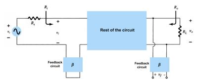
ii. Open-loop circuit diagram for voltage-shunt feedback
