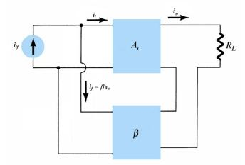
Current-shunt feedback amplifier is actually a closed-loop current-gain amplifier as shown below. We are going to find the derive the no-load gain  $A_{if}$ , input resistance  $R_{if}$  and output resistance  $R_{o\!f}$  of this closed-loop system.
