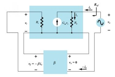
We can calculate the closed-loop output resistance (i.e., as a Thévenin equivalent resistance) by using the test voltage method as shown in the figure above. Note that as the feedback network is ideal, internal resistance of the feedback network is zero. So,  $v_x=0$  and  $v_o=i_1R_o+v_x=i_1R_o$ . Also as  $v_{if}=0$ ,  $v_i=-v_f=\beta i_o$ . Hence, output resistance  $R_{of}$
