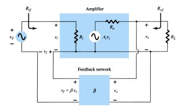
Let us derive no-load gain  $A_{vf}$ , input resistance  $R_{if}$  and output resistance  $R_{of}$  of the voltage-series feedback system in terms of the open-loop amplifier parameters  $A_v$ ,  $R_i$  and  $R_o$ .
