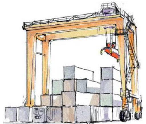
RTG crane (Rubber Tyre Gantry)
