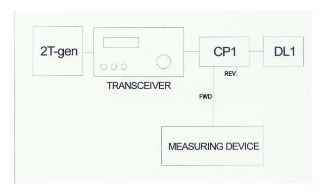
Several years ago, the most common measuring device was an oscilloscope or transmitter output monitor. While observing the transmitter output envelope, the 2-tone input was increased until "flat topping" was observed as an indication of transmitter compression. This procedure is well documented in older ARRL Handbooks. This procedure provides only an approximate indication of transmitter overload, but it is useful if more precise instruments are not available.
