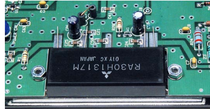
Figure 34. RF Board attached to the RF Power Module Screws.
