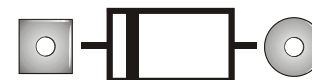
Figure 16. Circuit Board Diode Orientation Guides. The cathode always goes to the square solder pad on the board.
