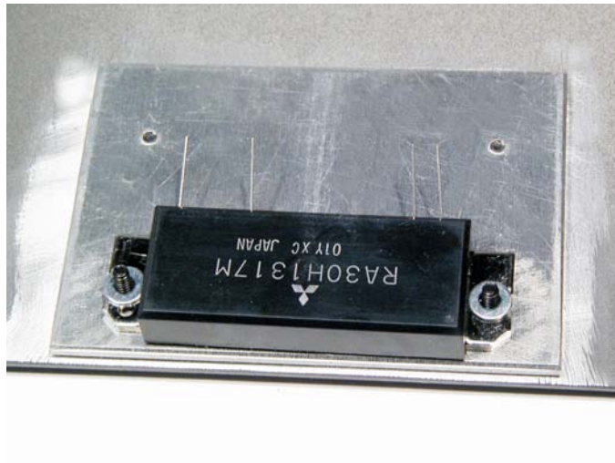
Figure 33. RF Power Module and Flat Washers in Place on the Heat Spreader.
