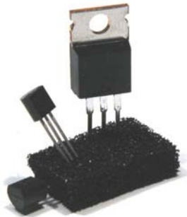
Figure 3. A common anti-static packaging is conductive foam which keeps all of the terminals of a device at the same potential.
