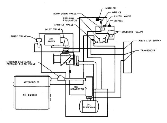
FIGURE 4b-1 - SCHEMATIC TUBING DIAGRAM
