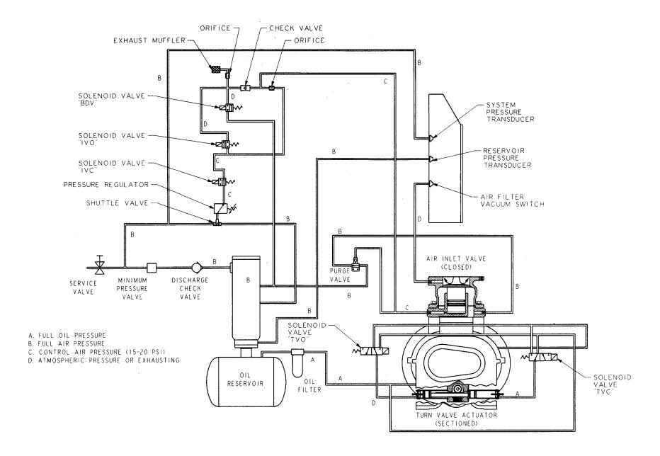
FIGURE 4b-8 - CONTROL SCHEMATIC - COMPRESSOR FULLY UNLOADED - CONSTANT SPEED MODE
