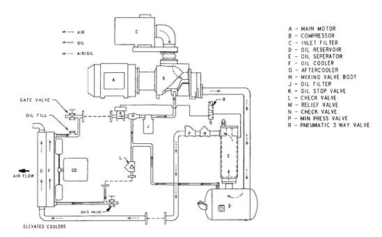
FIGURE 5-3 - OIL FLOW DIAGRAM REMOTE OVERHEAD MOUNTED
