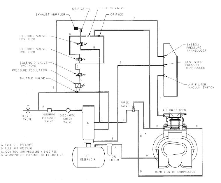
FIGURE 4a-7 - CONTROL SCHEMATIC - COMPRESSOR AT FULL LOAD
