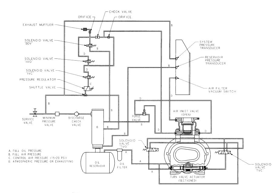
FIGURE 4b-7 - CONTROL SCHEMATIC - COMPRESSOR AT FULL LOAD
