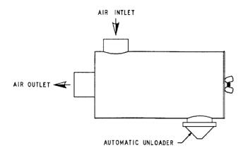
FIGURE 6-1 - HEAVY DUTY AIR FILTER (STANDARD)
