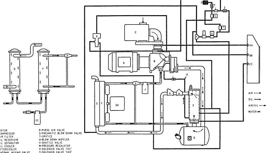
A-MOTOR B-COMPRESSOR C-AIR FILTER D-OIL RESERVOIR E-OIL SEPARATOR F-OIL COOLER G-AFTERCOOLER H-THERMAL MIXING VALVE J-OIL FILTER K-SEPARATOR TO CYLINDER OIL RETURN LINE L-CHECK VALVE M-PRESSURE RELIEF VALVE N-DISCHARGE CHECK VALVE P-MINIMUM DISCHARGE PRESSURE VALVE
