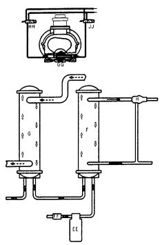
A-MOTOR B-COMPRESSOR C-AIR FILTER D-OIL RESERVOIR E-OIL SEPARATOR F-OIL COOLER G-AFTERCOOLER H-THERMAL MIXING VALVE J-OIL FILTER K-SEPARATOR TO CYLINDER OIL RETURN LINE L-CHECK VALVE M-PRESSURE RELIEF VALVE N-DISCHARGE CHECK VALVE P-MINIMUM DISCHARGE PRESSURE VALVE R-PURGE AIR VALVE
