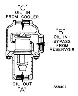
FIGURE 5-7 - THERMOSTATIC MIXING VALVE
