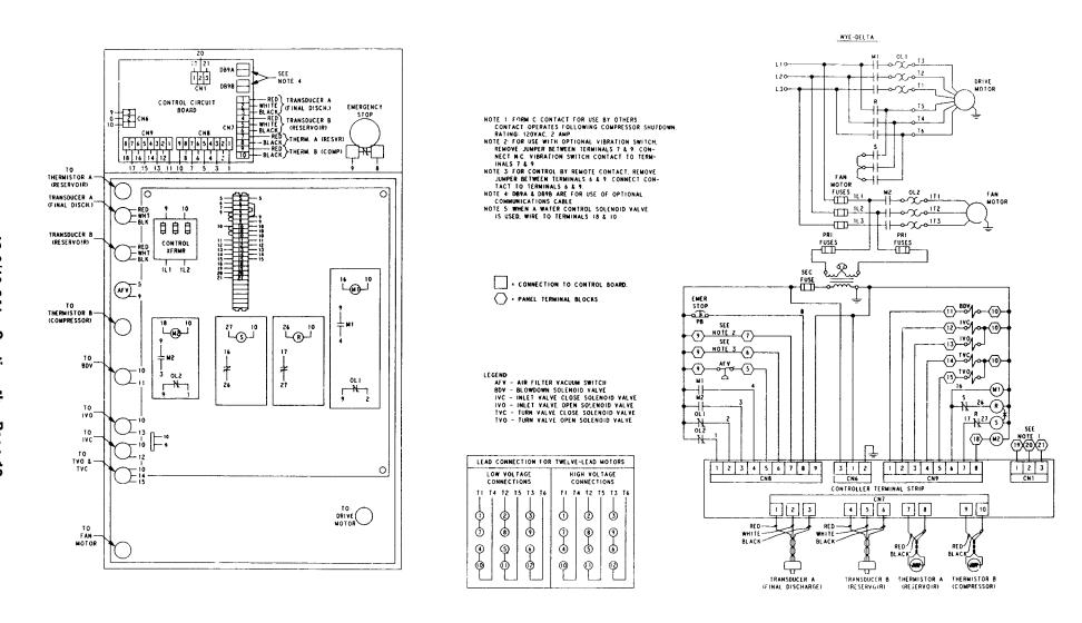
FIGURE 4b-10 - WIRING DIAGRAM - 208EAP546
