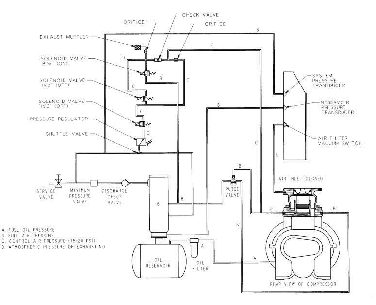
FIGURE 4a-6 - CONTROL SCHEMATIC - COMPRESSOR UNLOADED - CONSTANT SPEED MODE
