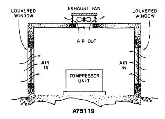
FIGURE 2-1 - TYPICAL COMPRESSOR ROOM
