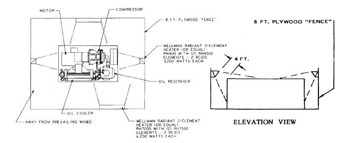
FIGURE 2-3 - COLD WEATHER INSTALLATION
