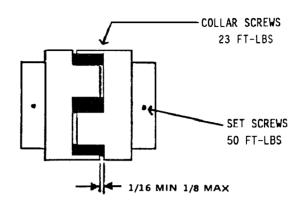
FIGURE 7-1 - INSTALLATION OF COUPLING CUSHIONS
