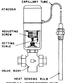
FIGURE 5-8 - WATER CONTROL VALVE
