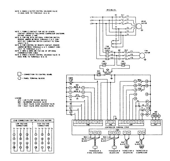
FIGURE 4a-9 - WIRING DIAGRAM - 207ECP546
