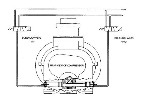
FIGURE 4b-5 - TURN VALVE ACTUATOR (SECTIONED)
