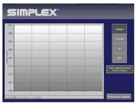
press the "Data Logging Disabled" button. When you are done, press the button again and the load bank will write the data in a tab-delimited format to the thumb drive.
