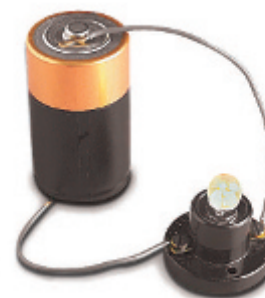
FIGURE 34.3 ▲ Each coulomb of charge that is made to flow in a circuit that connects the ends of this 1.5-volt flashlight cell is energized with 1.5 joules.
