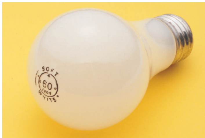
FIGURE 34.16 ▲ The power and voltage on the lightbulb read "60 W, 120 V." You can calculate the current that would flow through the bulb as follows: I = P/V = (60\text{ W})/(120\text{ V}) = 0.5\text{ A} .
