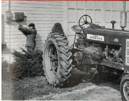
(Above) When the power line fails, just plug in Electrall to prevent financial loss and inconvenience. It supplies power to keep the farmstead fully electrified.
