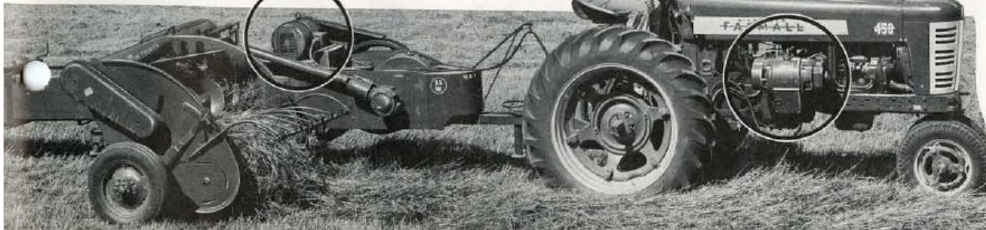
(Below) Electrall powered baler is started and stopped by an on-off switch. Electrall motor is completely enclosed and water-proof, readily transferred to other jobs.
