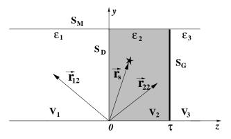
Fig. 3. Two-layered, terminated rectangular waveguide with an electric point source (starred) arbitrarily located in region  $V_2$  used in the magnetic-field formulation.
