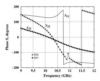
Fig. 8. Phase of the S-parameters versus frequency for the  $2 \times 3$  aperture-coupled patch array in the 7-port rectangular waveguide transition.
