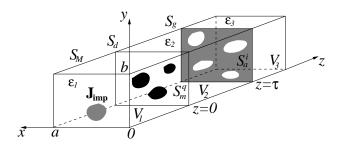
Fig. 1. Waveguide-based transition module of interacting electric- (patch, strip) and magnetic-type (slot, aperture) discontinuities.
