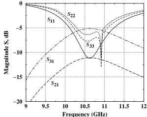
Fig. 7. Magnitude of the S-parameters versus frequency for the  $2 \times 3$  aperture-coupled patch array in the 7-port rectangular waveguide transition.
