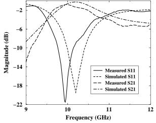
Fig. 6. Numerical and experimental results for the reflection and transmission coefficient of the single unit cell, including a waveguide-based aperture-coupled patch antenna and a waveguide-to-microstrip line junction.
