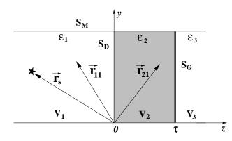
Fig. 2. Two-layered, terminated rectangular waveguide with an electric point source (starred) arbitrarily located in region  $V_1$  used in the electric-field formulation.
