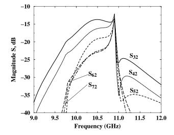
Fig. 10. Port-to-port coupling in the  $2 \times 3$  aperture-coupled patch array.
