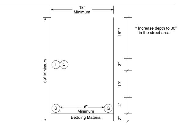
Figure 2-6 Typical Joint Service Trench
