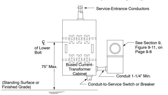
Figure 7-11 Overhead-Fed, Separate-Bused, Current-Transformer Cabinet and Safety-Socket Meter Box (201 Amps–400 Amps, 3∅, and 201 Amps–600 Amps, 1∅)
