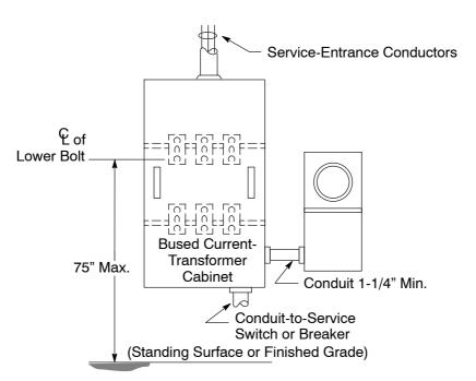
Figure 6-10 Overhead-Fed, Separate-Bused, Current-Transformer Cabinet and Meter Box (401 Amps and Above)
