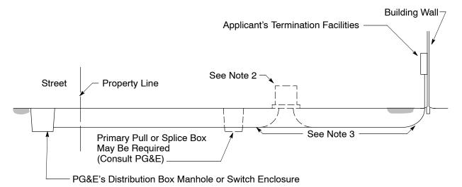
Figure 3-2 Underground-to-Underground Service Connection
