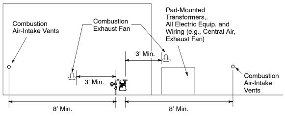
Figure 2-22 Gas Regulator Set Spatial Clearance Requirement from Sources of Ignition
