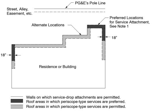
Figure 4-1 Preferred and Alternate Locations for the Overhead Service Drop Attachment (see Note 2)
