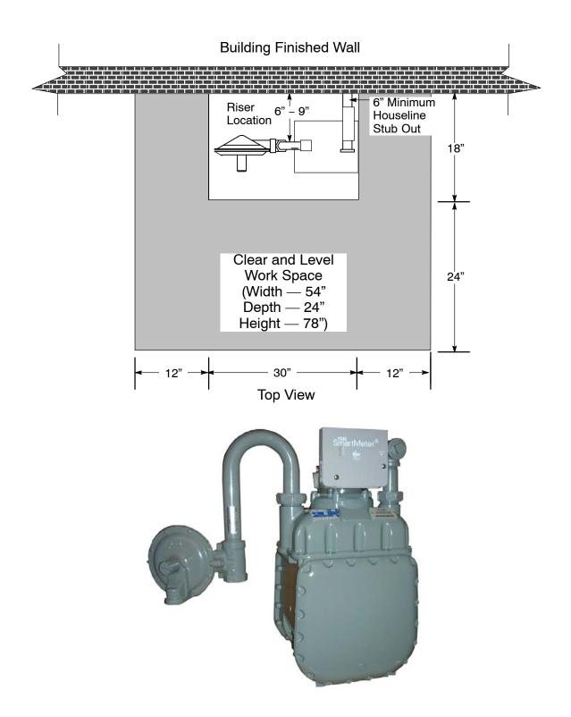
Figure 2-16 Typical Gas Meter Connection for 400 to 1000 Class Meter
