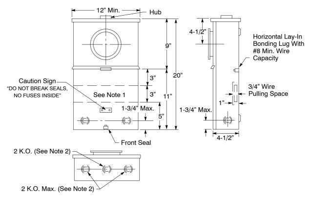
Figure 9-11 Meter Box for Transformer-Rated Metering (for Single-Phase or Three-Phase Installations)
