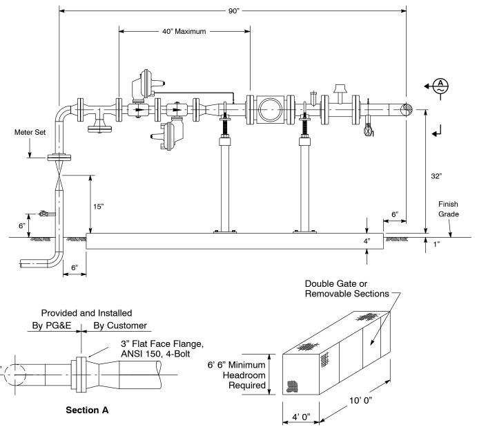
4. Figure 2-18 represents a rotary gas meter with 3,001 through 7,000 scfh at an approved delivery pressure.
