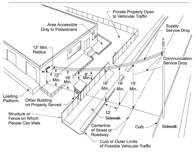
Figure 4-12 Ground Clearances for Supply Service Drops, 0 Volts Through 750 Volts, Industrial and Commercial Installations (Required by the CPUC)
