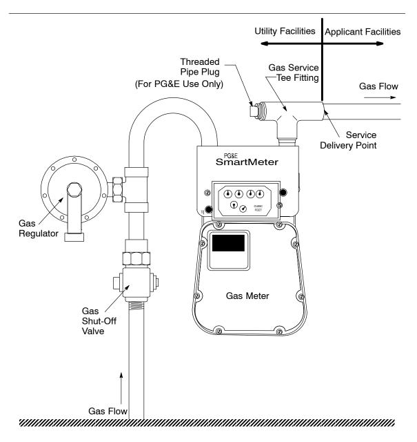
Figure 2-28 Typical Residential/Small Commercial Meter
