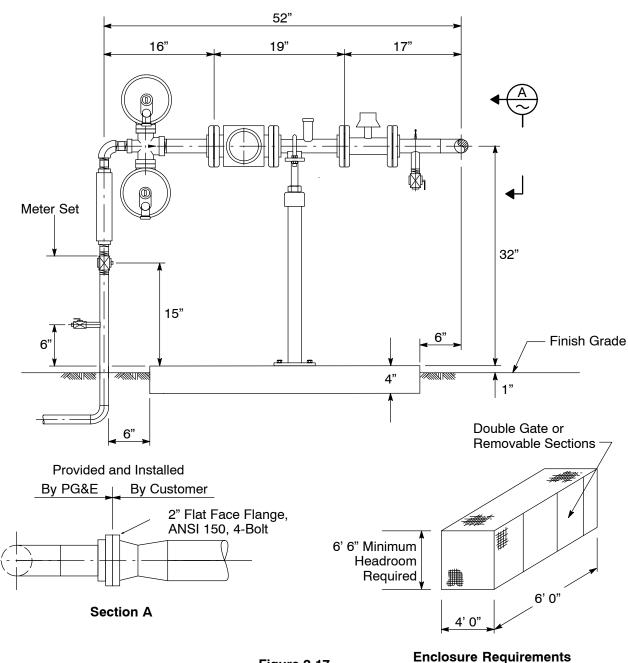
3. Figure 2-17 represents a rotary gas meter with 1,401 through 3,000 scfh at an approved delivery pressure.
