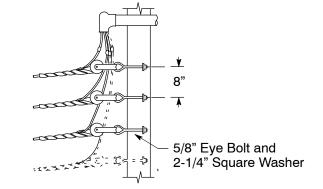
Figure 4-31 Service Drop Cable, 4/0 and Smaller, Triplex or Quadruplex
