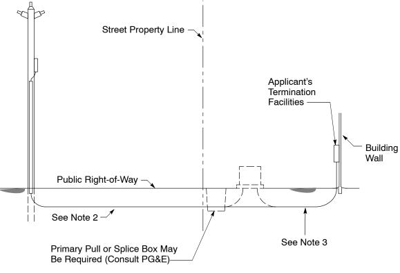
Figure 3-3 Overhead-to-Underground Service Connection
