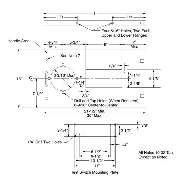
Figure 10-25 Standard Switchboard Service Section, 15-Inch Hinged Panel for Socket Meter
