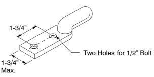
Figure 9-16 Service-Terminal Conductor Connector
