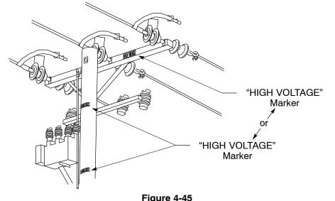
Figure 4-45 High-Voltage Marker on Poles and Crossarms
