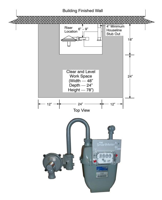
Figure 2-15 Typical Residential Gas Meter Connection
