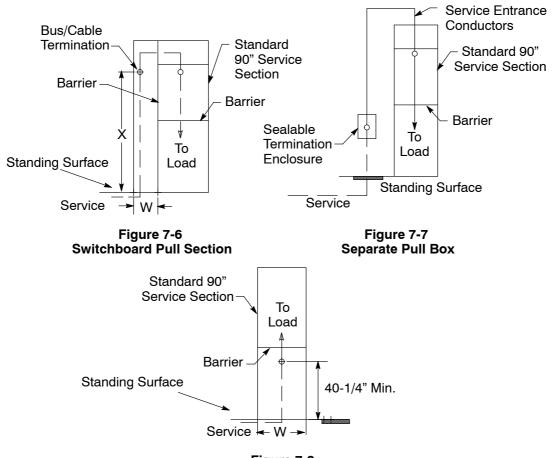
Figure 7-8 Bottom-Fed Service Section
