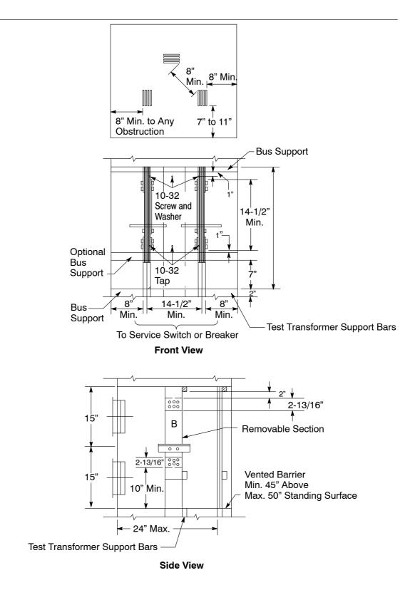
Figure 10-5 Standard Switchboard, CT Compartment, 3,001 Amps and Larger, Three-Phase, 3-Wire Service
