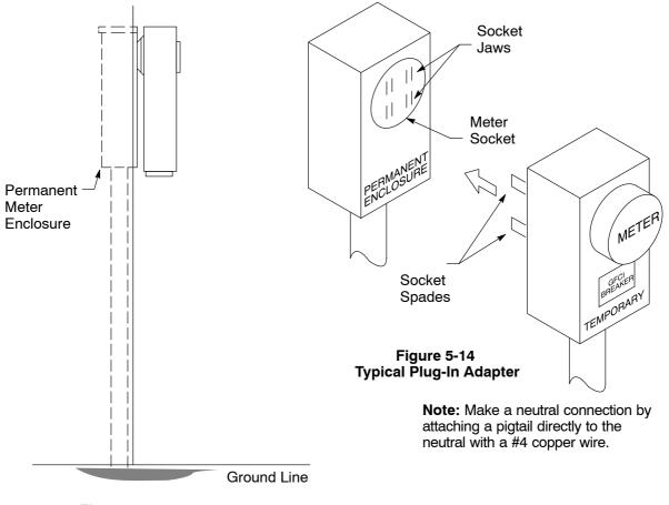
Figure 5-13 Plug-In Temporary Service
