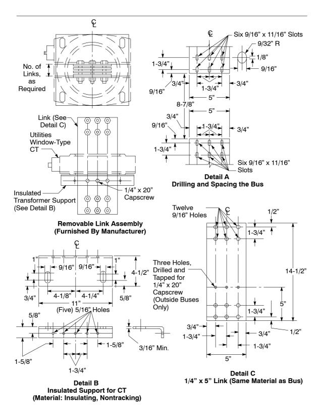
Figure 10-10 Switchboards, 0 Volts–600 Volts, CT Compartment, Removable Link and CT Support (Six-Bolt Configuration)
