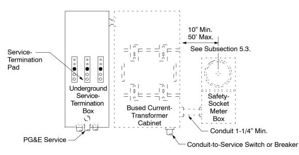
Figure 6-5 Typical Underground, Separate-Bused, Current-Transformer Cabinet and Safety-Socket Meter Box Assembly, 120/240-Volt, 400-Amp Through 600-Amp Service
