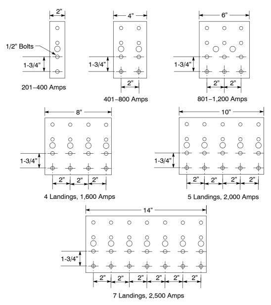
Figure 9-15 Detail of Aluminum, Termination Bus Stubs
