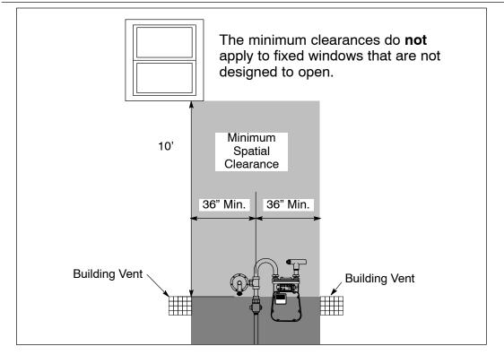
Figure 2-21 Gas Meter Set Spatial Clearance From Building Openings, Vents, and Windows
