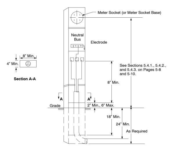
Figure 6-1 Residential Electric Metering Pedestal
