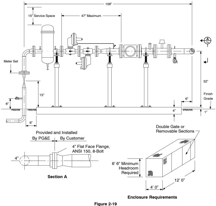
Gas Meter Connection Using an 11M or 16M Rotary Gas Meter
