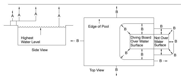
Figure 4-3 Minimum Clearance for All Drops Above or Adjacent To Swimming Pools
