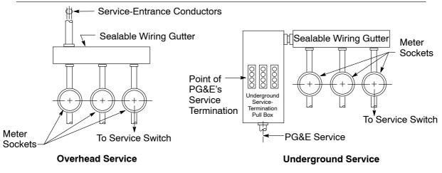
Figure 6-11 Meter Sockets With Wiring Gutters
