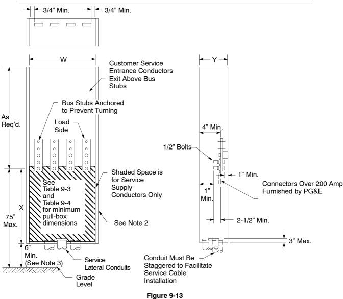
Typical Underground Service Termination Section and Pull Box, Wall-Mounted or Pad-Mounted (Floor-Standing)
