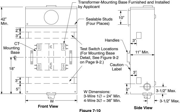
Overhead-Fed Combination Meter and Current-Transformer Cabinet, (201 Amps–400 Amps, 3∅ and 201 Amps–600 Amps, 1∅)
