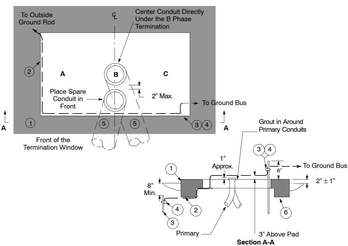
Figure 11-1 Primary Switchboard Termination Section Pad Detail
