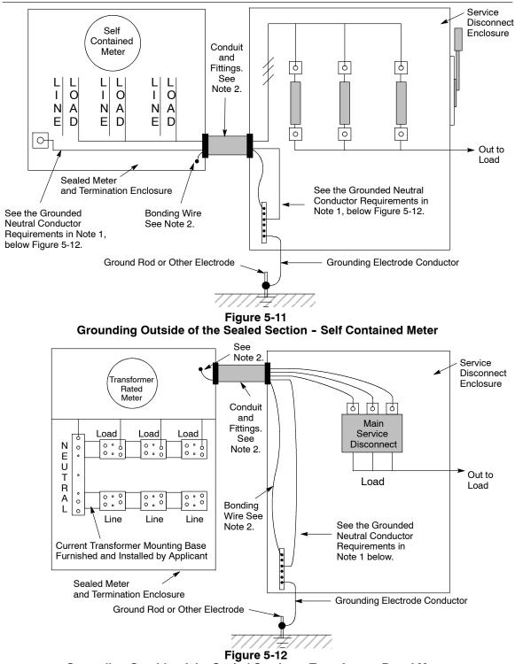
Grounding Outside of the Sealed Section - Transformer Rated Meter
