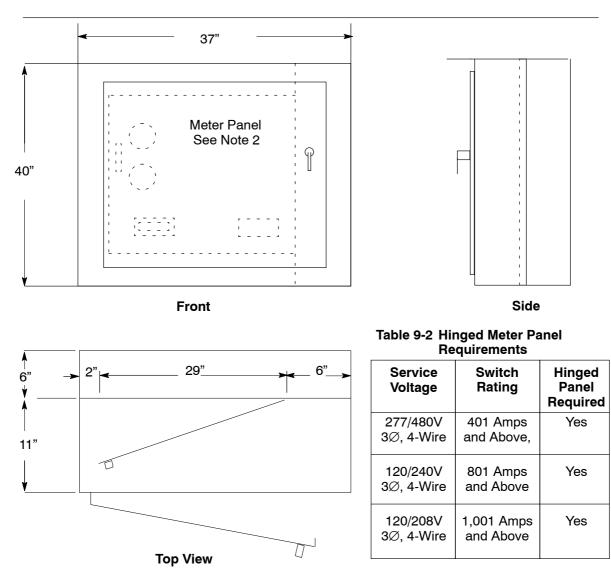
Figure 9-12 Remote Metering Cabinet (for Three-Phase Installations)
