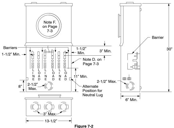
Bused, Safety-Socket Meter Box for Self-Contained Metering (126 Amps-225 Amps)
