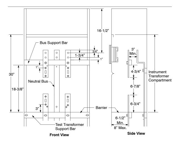
Figure 10-1 Standard Switchboard, CT Compartment, 0 Amps–1,000 Amps, Single-Phase or Three-Phase, 3-Wire Service
