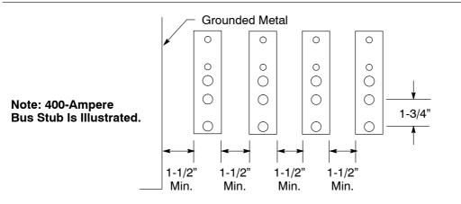
Figure 9-14 Detail of Clearance Requirements for Adjacent Termination Bus Stubs
