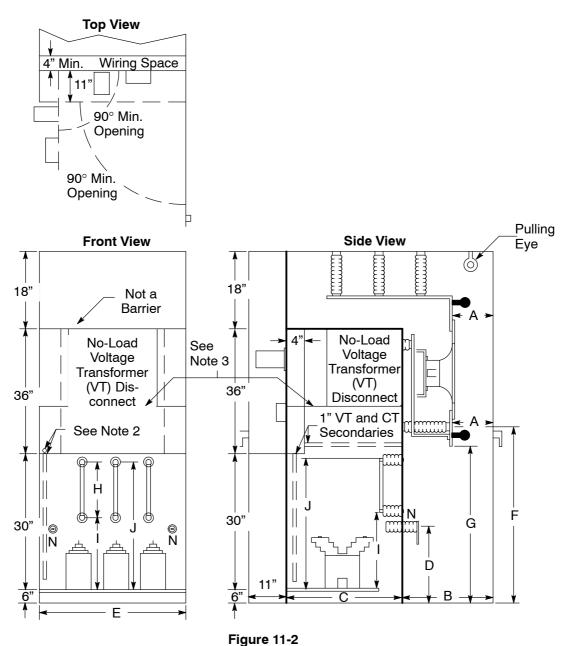
Typical, High-Voltage Metering Enclosure: 2,400-Volt Through 17,000-Volt Service
