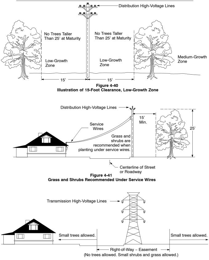
Figure 4-42 Grass and Shrubs Recommended Under Transmission Wires
