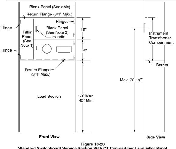
Standard Switchboard Service Section With CT Compartment and Filler Panel, 0 Volts-600 Volts
