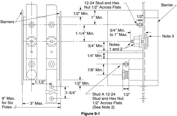
Test Blocks for Self-Contained Metering, 0 Amps-225 Amps
