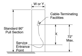
Figure 10-16 Switchboard Pull Section Front View (Y-Side, Low Entry), Side View (W-Back, Low Entry)
