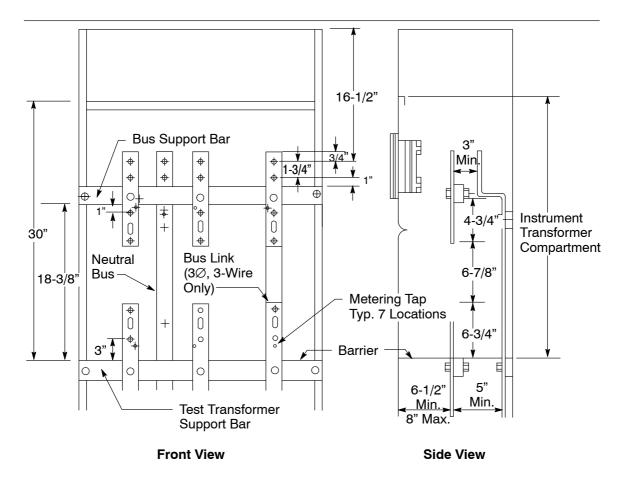
Figure 10-2 Standard Switchboard, CT Compartment, 0 Amps–1,000 Amps, Three-Phase, 3-Wire and 4-Wire Services
