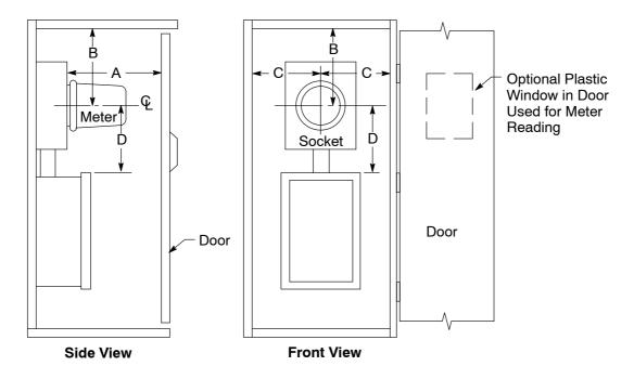
Figure 5-2 Meter Cabinet Enclosure Clearances
