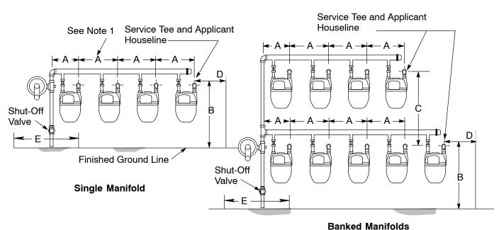
Figure 2-23 Dimensions for Typical, Residential, Multimeter Installations
