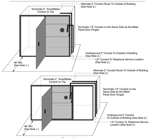
Figure 5-1 Preferred Location of Conduits for Indoor and Outdoor Meter Panels and Switchboards
