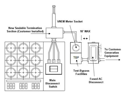
Figure 3(b): Point of Connection for Overhead Service
