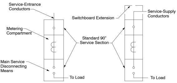
Figure 7-12 Overhead, Service-Termination, Standard Switchboard Service Section (0 Volts–600 Volts)
