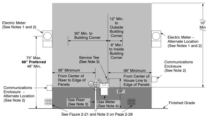
Figure 2-20 Electric and Gas Meter Set Separation Dimensions and Clearances
