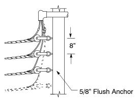
Figure 4-33 New or Existing Wall, 1/0 kcmil <sup>1</sup> to 397.5 kcmil Aluminum
