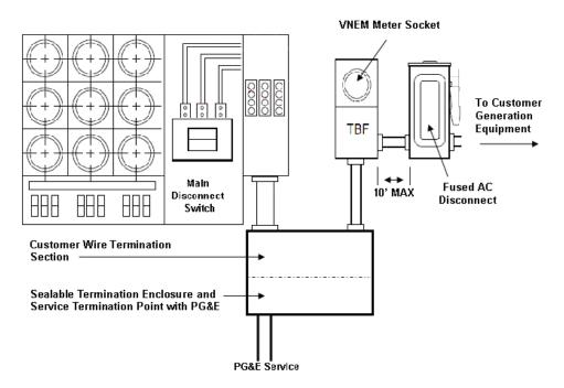
Figure 2(b): Point of Connection with Termination Enclosure for Underground Service
