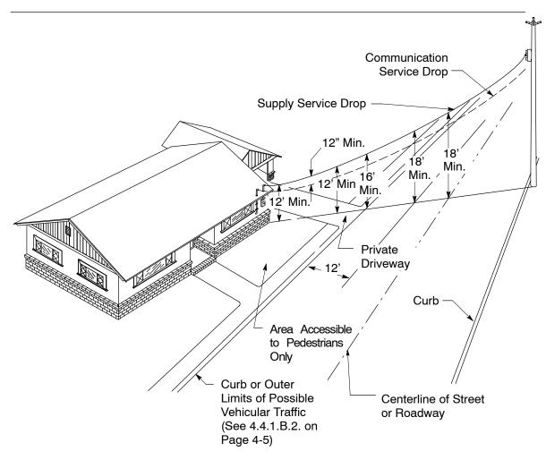
Figure 4-2 Ground Clearances for Supply Service Drops, 0 Volts Through 750 Volts, Residential Installations (Required by the CPUC)
