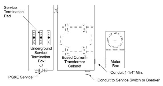
Figure 7-5 Separate-Bused Current-Transformer Cabinet and Meter Box With Underground Service-Termination Pull Box (201 Amps–400 Amps, 3∅ and 201 Amps–600 Amps, 1∅)
