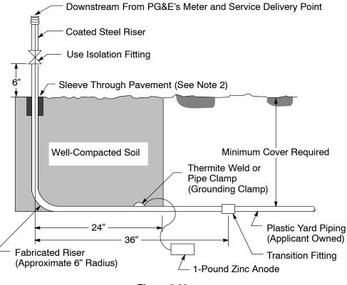
Figure 2-29 Recommended, Applicant-Owned Riser and Pipe
