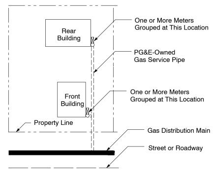
Figure 2-7 Separate Gas Services for Two Buildings on a Single Lot
