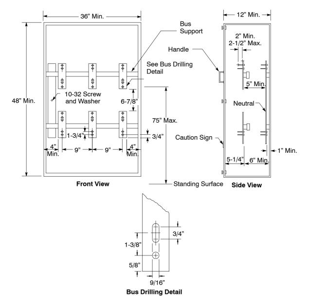
Figure 9-10 Bused CT Cabinet (4-Wire Service, 201 Amps-800 Amps)
