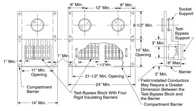
Figure 10-11 Standard Section for Self-Contained Meter Sockets, 0 Amps–225 Amps, Installed in Switchboards: Nonresidential
