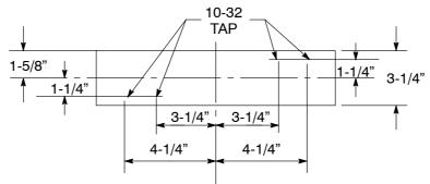
Figure 9-2 Removable Test Switch Mounting-Base Detail
