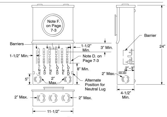
Figure 7-1 Bused, Safety-Socket Meter Box for Self-Contained Metering (0 Amps–125 Amps)
