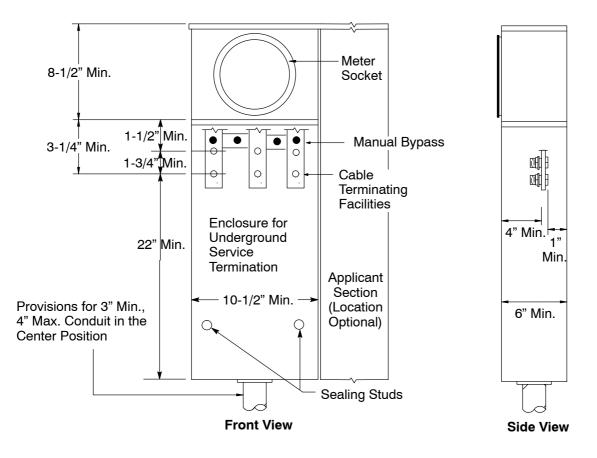
Figure 6-3 Typical Service-Termination Enclosure, Combination Meter-Socket Panel for a Class 320 Meter (Residential/Commercial, 120/240-Volt, 226-Amp Through 320-Amp Service)
