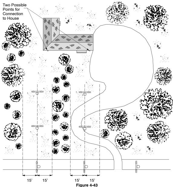
Alternative Routes to a House Showing High-Voltage Lines and Tree-Clearance Zones
