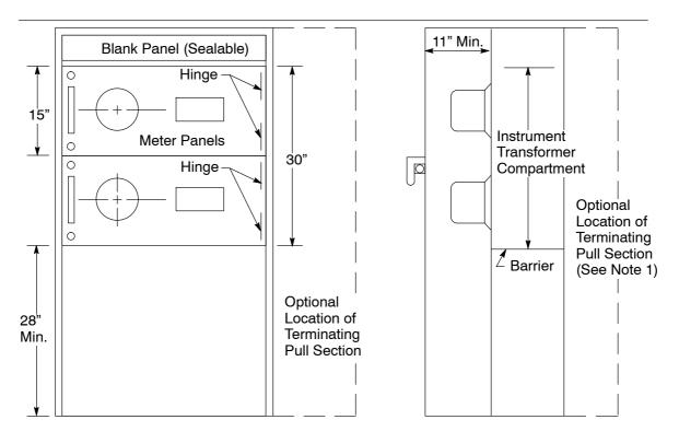
Figure 10-24 Low-Profile Switchboard Service Section With CT Compartment for Underground, Outdoor Application, 0 Volts–600 Volts
