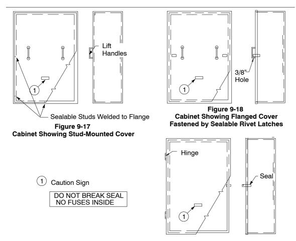
Figure 9-19 Cabinet Showing Hinged, Flanged Cover
