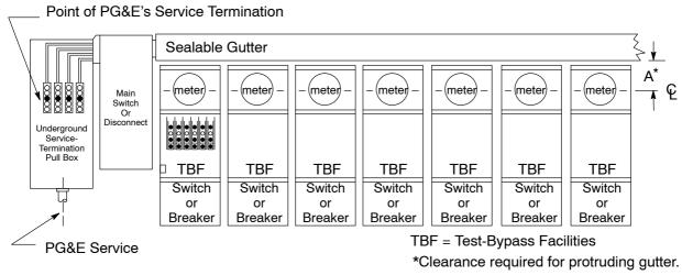
Figure 7-15 Grouped-Meter Installation *With* a Main Switch
