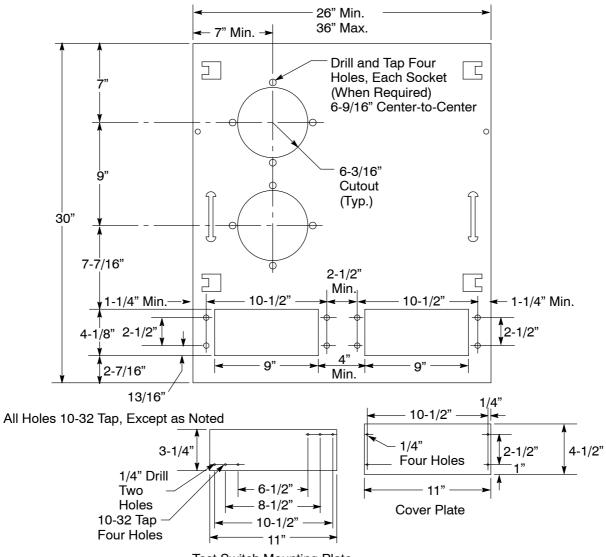
Test Switch Mounting Plate
