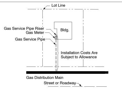
Figure 2-1 Typical Gas Service Installation
