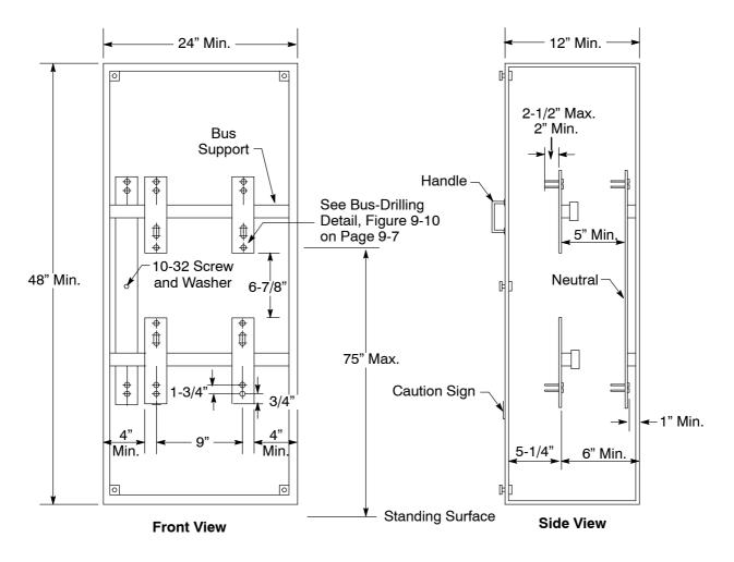
Figure 9-9 Bused CT Cabinet, 3-Wire Service, 201 Amps-800 Amps
