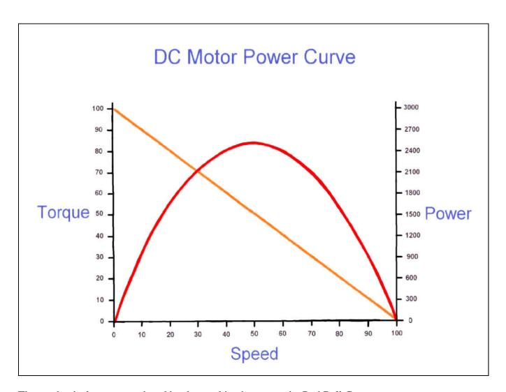
The mechanical energy produced by the machine is seen as the Red Bell Curve.
