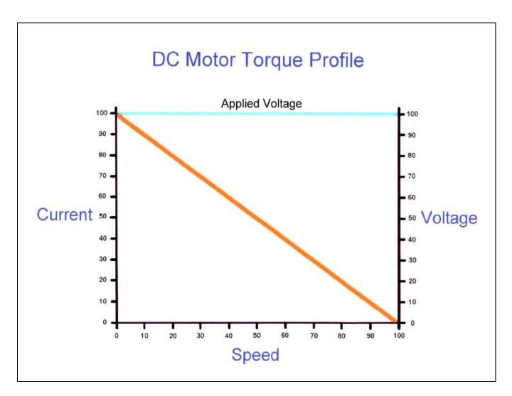
Here is the graph that depicts the torque produced by the machine. With a steady Applied Voltage, the torque produced follows the same characteristics as the Current.
