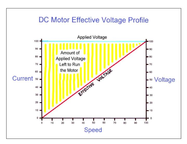
Conversely, this is the diagram that depicts the Effective Voltage Profile. It is what is left when the Back EMF is subtracted from the Applied Voltage.
