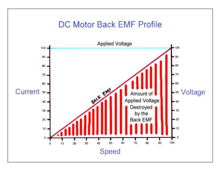
So, just to review, here is a diagram of the Back EMF profile of one of our Permanent Magnet Field DC Motors.
