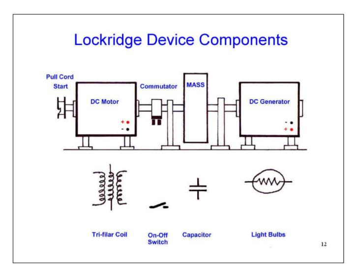
So, here again is the list of components for the Lockridge Device, but this time, in graphical form.
