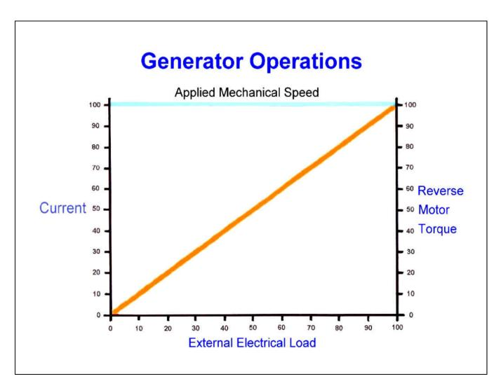
Here is a graph showing the Generator Operations. At any given applied mechanical speed, the production of current to power external loads is in direct proportion to the activation of the reverse motor torque which makes the generator harder to turn.
