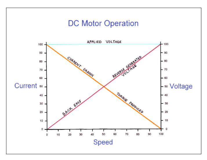
So, here is our boring little drawing again, and now we can see what it really means. The machine is always both a motor and a generator.
