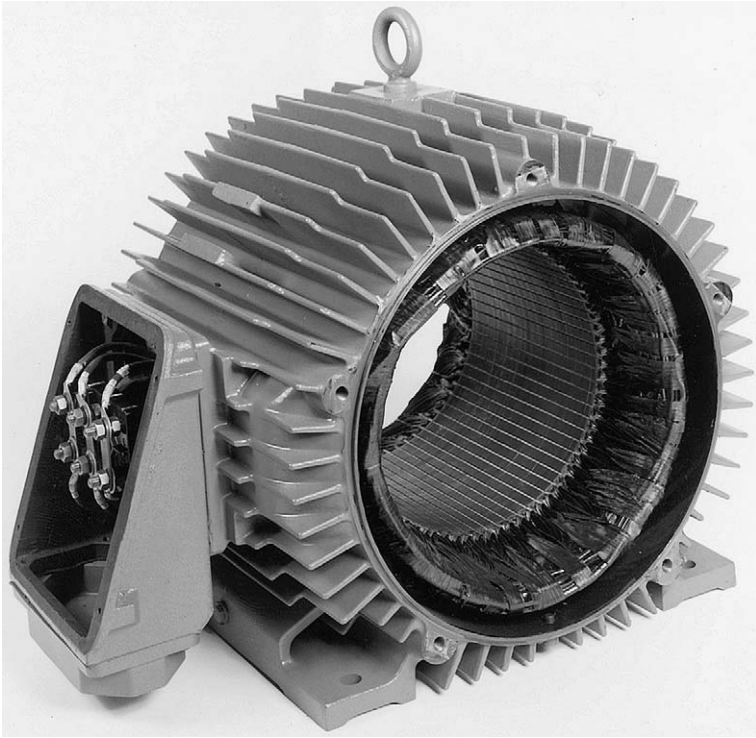
Plate 5.1 Stator of three-phase induction motor. The semi-closed slots of the stator core obscure the active sides of the stator coils, but the ends of the coils are just visible beneath the binding tape. (Photograph by courtesy of Brook Crompton)
