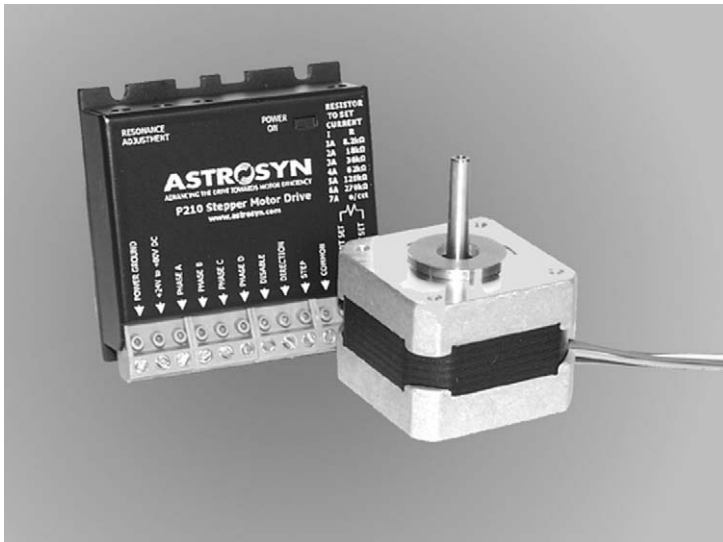
Plate 9.4 Bipolar constant-current chopper drive with size 17 hybrid motor. This versatile drive draws its power from a d.c. supply (between 24 V and 80 V) and the output phase current can be set (using programming resistors) to any value in the range 0.3 A to 7 A. A resonance adjustment is provided. (Photo courtesy of Astrosyn)
