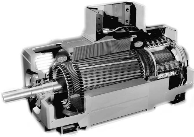
Plate 3.1 Cutaway view of 4-pole d.c. motor. The skewed armature windings on the rotor are connected at the right-hand-end via risers to the commutator segments. There are four sets of brushes, and each brush arm holds four brush-boxes. The sectioned coils surrounding two of the four poles are visible close to the left-hand armature end-windings. (Photo courtesy of ABB)
