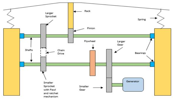
Figure 7.1 Constructional details of Electro-mechanical unit
