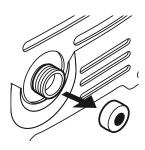
2. Attach the Gun/Extension Nozzle holder to the side of the body.
