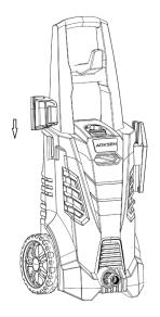
3 Attach the Cable Holder to the side of the body
