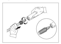
2. Press release button on bottom of gun toward back of the gun, then insert high pressure hose.
