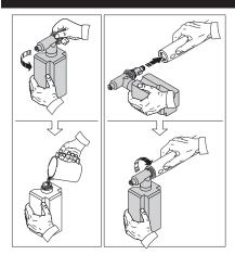
The use of detergents can dramatically reduce cleaning time and assist in the removal of difficult stains. Some detergents have been customized for pressure washer use on specific cleaning tasks. These detergents are approximately as thick as water. The use of thicker detergents, such as dish soap, will clog the chemical injection system and prevent the application of the detergent.
