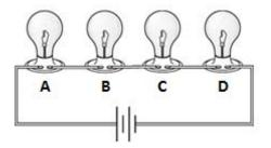
Because some voltage is "used up" by each bulb in the circuit, each additional bulb means the voltage is divided among more bulbs and is therefore less for each bulb. This is why light bulbs get dimmer as you add more bulbs in series.
