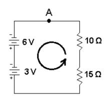
If we start at point A and move counterclockwise around the loop (in the direction of the arrow), the voltage should be zero when we get back to point A.
