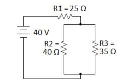
Because the circuit has series and parallel sections, we cannot simply use the series and parallel rules across the entire table.
