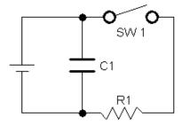
Which of components C1 and SW1 are in series with R1? Which are in parallel with R1?
