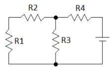
Which resistors are in series with R1? Which are in parallel with R1?
