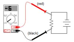
The reading of -6V indicates that the potential difference is 6V, but the current is actually flowing in the opposite direction from the way the voltmeter is measuring—from the black (-) lead to the red (+) lead.
