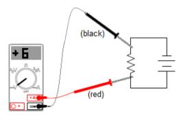
If you switch the leads, so the black (-) lead is on the more positive end and the red (+) lead is on the more positive end, the voltage reading would be negative. In this circuit, the voltmeter reads -6V:
