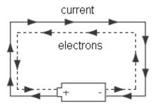
This means that electric current "travels" in the *opposite* direction from the electrons.
