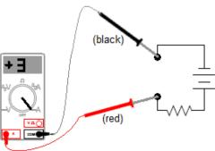
As with the voltage example above, if you switched the leads, the reading would be -3A instead of +3A.
