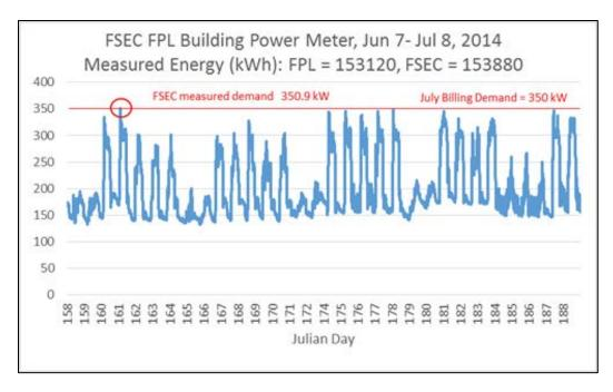
Figure 3. Comparison of FPL Billing Information to FSEC Measured Energy Use and Facility Demand
