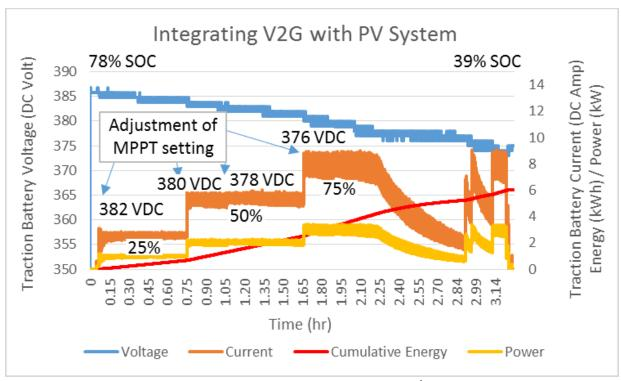
Figure 7. System Parameters during V2G w/PV Testing
