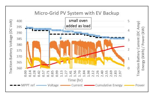
Figure 9. System Parameters during Micro-Grid Testing
