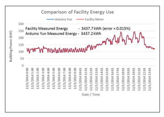
Figure 4. Comparison of Facility Measured Energy and Parallel Measurement
