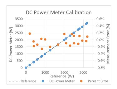
**Figure 5. Laboratory Meter Calibration Results**
