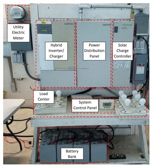
Figure 6. Photovoltaic Training Panel and Hardware
