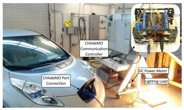
Figure 8. Operational Micro-grid Application using Electric Vehicle
