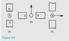
The direction of the e.m.f., and thus the current due to the e.m.f. may be obtained by either Lenz's law or Fleming's Right-hand rule (i.e. GeneRator rule).
