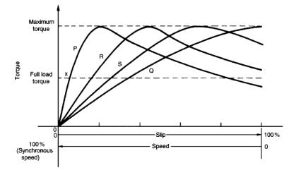
speed variation with variations of load. Curves R and S of Fig. 23.9 are characteristics for values of rotor resistance's between those of P and Q. Better starting torque than for curve P is obtained, but with lower efficiency and with speed variations under operating conditions.
