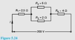
(a) The equivalent resistance  $R_x$  of  $R_2$  and  $R_3$  in parallel is:
