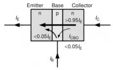
(a) n-p-n bipolar junction transistor
