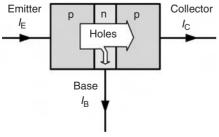
(b) p-n-p bipolar junction transistor
