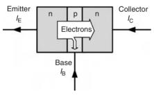
(a) n-p-n bipolar junction transistor
