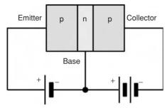
(b) p-n-p bipolar junction transistor
