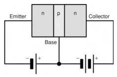
(a) n-p-n bipolar junction transistor
