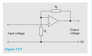
The op amp shown in Fig. 19.9 is a non-inverting amplifier, similar to Fig. 19.8
