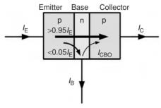
(b) p-n-p bipolar junction transistor
