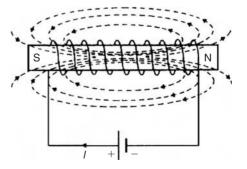
(b) Magnetic field of an iron cored solenoid
