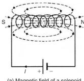
(a) Magnetic field of a solenoid
