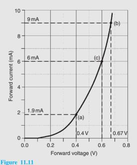
(a) From Fig. 11.11, when  $V = 0.4 \,\text{V}$ , current flow $ing, I = 1.9 \, mA$
