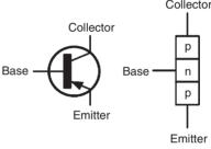
(b) p-n-p bipolar junction transistor (BJT)
