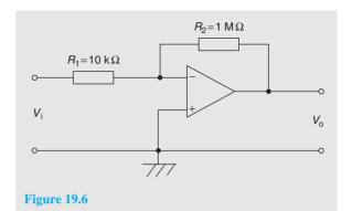
Comparing Fig. 19.6 with Fig. 19.5, gives  $R_i = 10 \text{ k}\Omega$ and  $R_{\rm f} = 1 \, {\rm M}\Omega$
