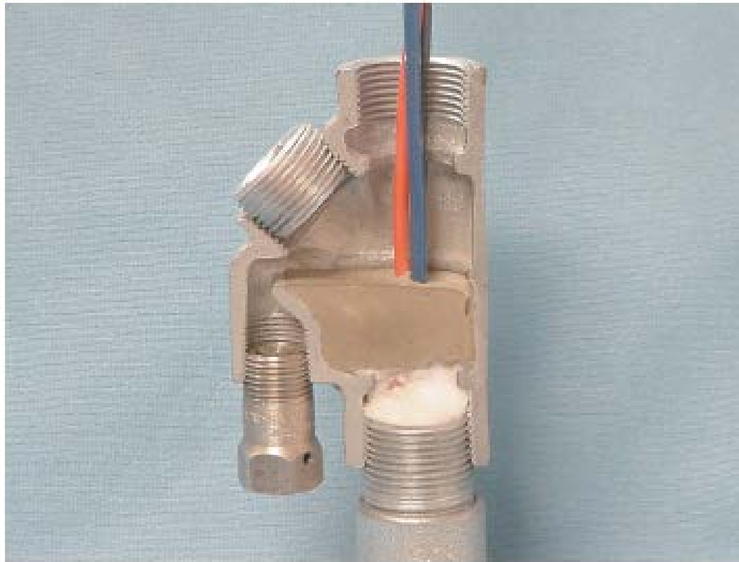
Exhibit 501.9 A sealing fitting placed in a run of conduit to minimize the passage of gases from one portion of the electrical installation to another. (Courtesy of Appleton Electric Co., EGS Electrical Group)
