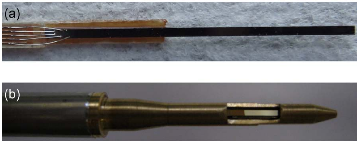
Figure C.1: Mounted W-band EDMR sample. (a) Wirebonded EDMR chip on PCB support piece. (b) Sample inserted into extractable W-band probe tip.
