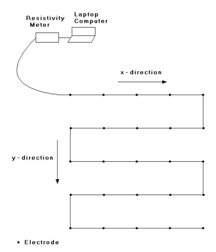
Figure 29. The arrangement of the electrodes for a 3-D survey.
