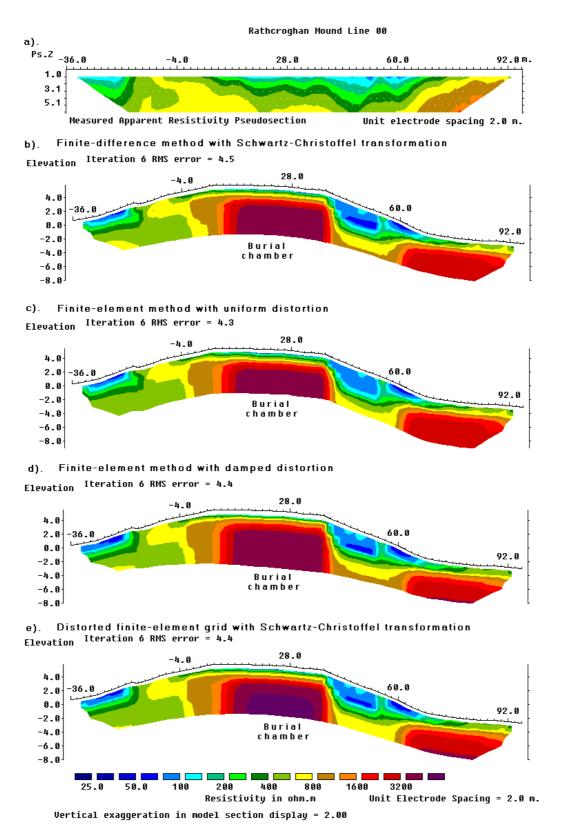
Figure 40. Inversion models for the Rathcroghan Mound data set. (a) Measured apparent resistivity data set. Models obtained using (a) the Schwartz-Christoffel transformation method using a finite-difference mesh (b) finite-element method with uniform distortion (c) finite-element method with damped distortion (d) finite-element method with the distortion calculated using Schwartz-Christoffel transformation for the topography modelling.
