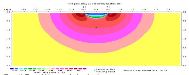
Figure 11. The sensitivity pattern for the pole-pole array.
