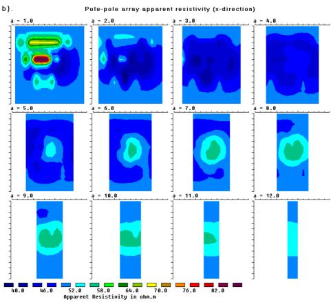
Figure 32. (a) 3-D model with 4 rectangular blocks and a 15 by 15 survey grid. (b) Horizontal apparent resistivity psudosections for the pole-pole array with the electrodes aligned in the x-direction.
