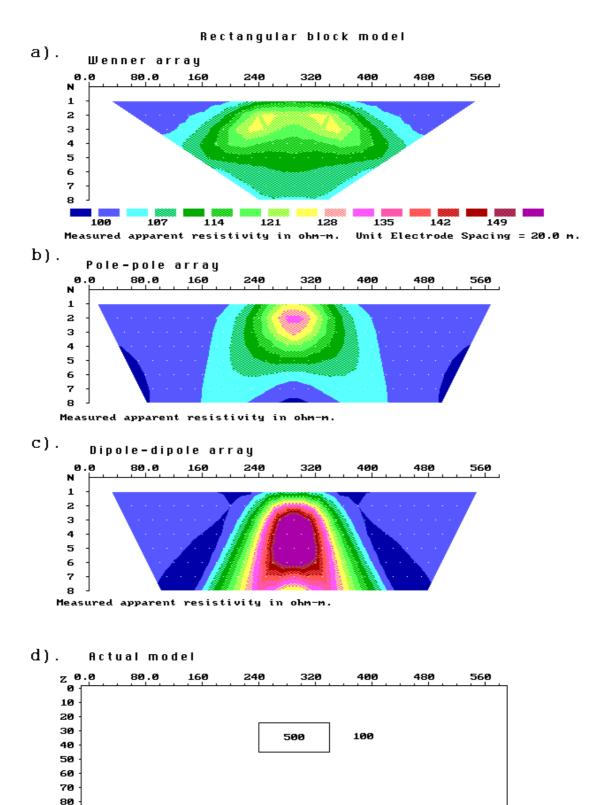
Figure 7. The apparent resistivity pseudosections from 2-D imaging surveys with different arrays over a rectangular block.
