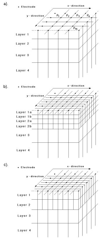
Figure 33. The models used in 3-D inversion. (a) Standard model where the widths of the rectangular blocks are equal to the unit electrode spacings in the x- and y-directions. (b) A model where the top few layers are divided by half, both vertically and horizontally, to provide better resolution. (c) A model where the model blocks are divided in the horizontal directions but not in the vertical direction.
