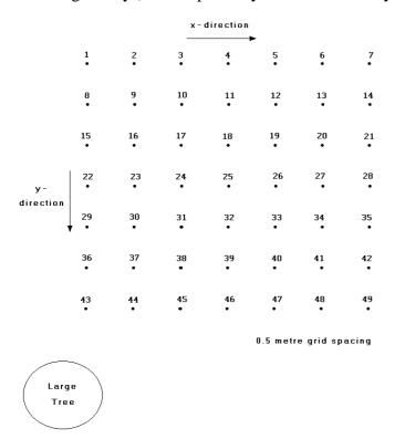
Figure 34. Arrangement of electrodes in the Birmingham 3-D field survey.
