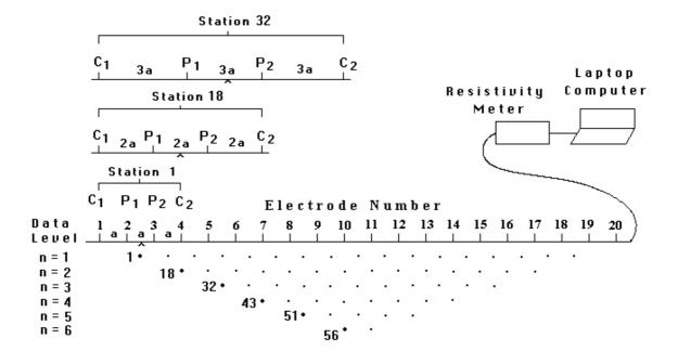
Figure 5. The arrangement of electrodes for a 2-D electrical survey and the sequence of measurements used to build up a pseudosection.
