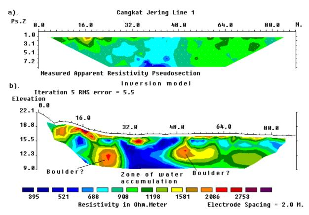
Figure 19. (a) The apparent resistivity pseudosection for a survey across a landslide in Cangkat Jering and (b) the interpretation model for the subsurface.
