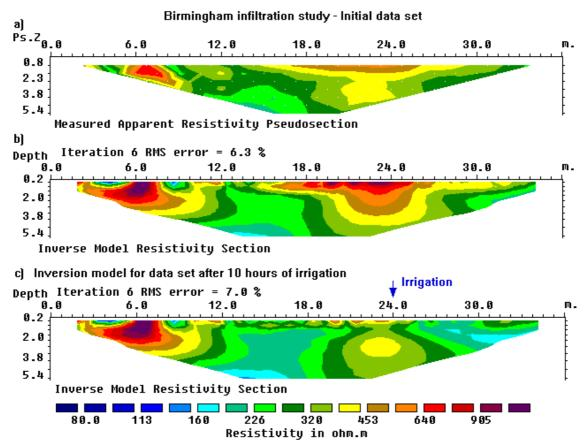
Figure 24. (a) The apparent resistivity and (b) inversion model sections from the survey conducted at the beginning of the Birmingham infiltration study. This shows the results from the initial data set that forms the base model in the joint inversion with the later time data sets. As a comparison, the model obtained from the inversion of the data set collected after 10 hours of irrigation is shown in (c).
