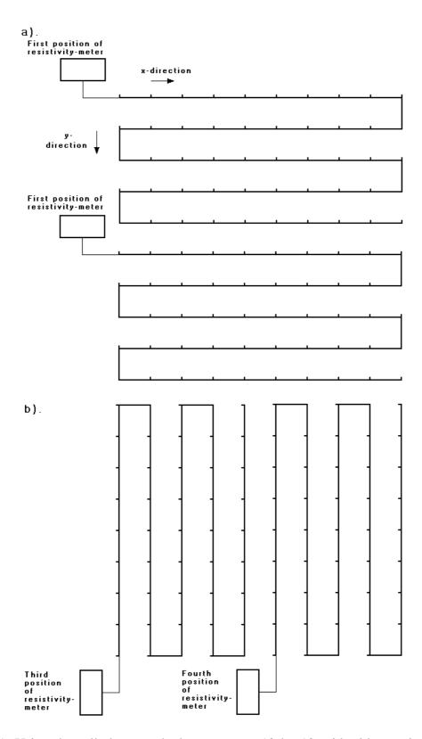
Figure 31. Using the roll-along method to survey a 10 by 10 grid with a resistivity-meter system with 50 electrodes. (a) Surveys using a 10 by 5 grid with the lines orientated in the x-direction. (b) Surveys with the lines orientated in the y-direction.
