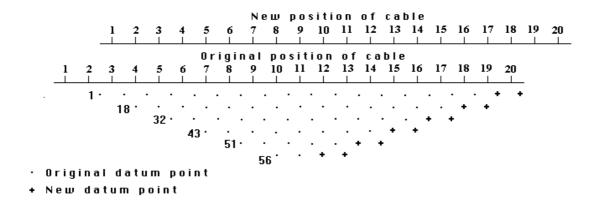
Figure 6. The use of the roll-along method to extend the area covered by a survey.
