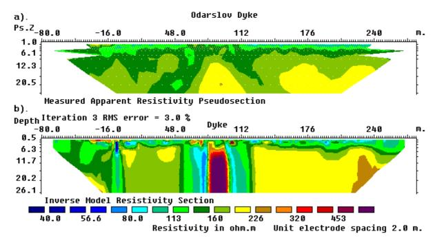
Figure 17. The observed apparent resistivity pseudosection for the Odarslov dyke survey together with an inversion model.
