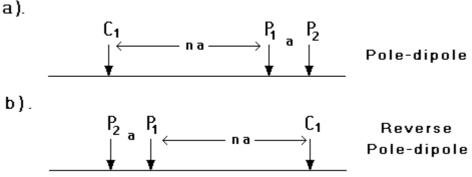
Figure 12. The forward and reverse pole-dipole arrays.
