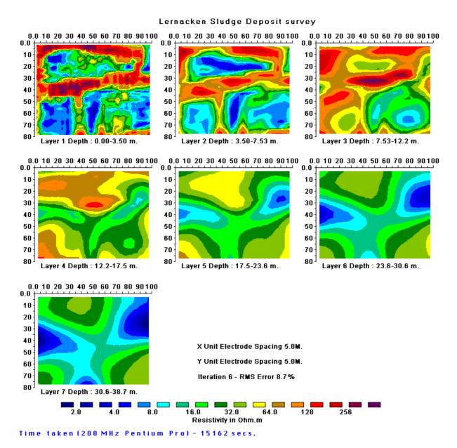
Figure 37. The 3-D model obtained from the inversion of the Lernacken Sludge deposit survey data set displayed as horizontal slices through the earth.
