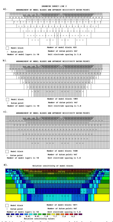
Figure 15. Subdivision of the subsurface into rectangular blocks to interpret the data from a 2-D imaging survey using different algorithms. Models obtained with (a) the default algorithm, (b) by allowing the number of model blocks to exceed the number of datum points, (c) a model which extends to the edges of the survey line and (d) using the sensitivity values for a homogeneous earth model.
