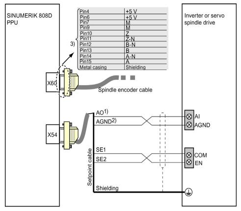
Figure 3-4 Connecting the inverter or the servo spindle drive (bipolar)
