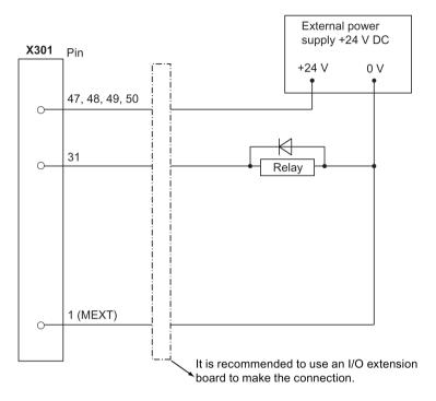
To supply the digital outputs, you must connect an external 24 V DC power supply (X301, X302: pins 47, 48, 49, 50).
