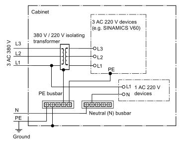
Note that the PE/PEN busbar in the cabinet must connect to the ground through a grounding cable with a cross section  $\geq$  10 mm<sup>2</sup> as illustrated below.
