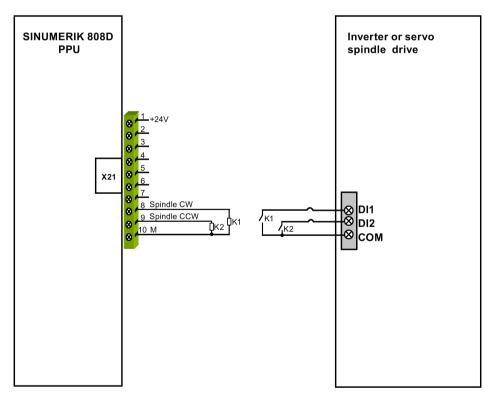
NC readiness is in the form of a relay contact (NO). It must be integrated into an EMERGENCY STOP circuit. The connection diagram is shown as follows:
