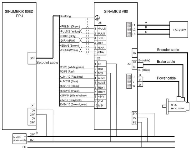
1): If necessary, you can also serially connect an emergency stop switch between the 65 enable signal and the 24V signal.
