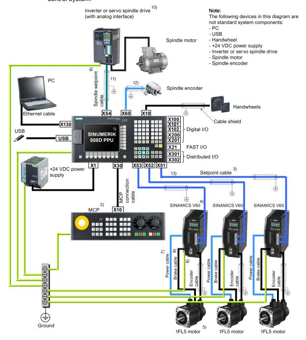
11), 12): For detailed information on cable shield connection, refer to Section "Analog spindle interface - X54 (Page 33)".13): For detailed information on cable shield connection, refer to Section "Pulse drive interfaces - X51, X52, X53 (Page 30)".
