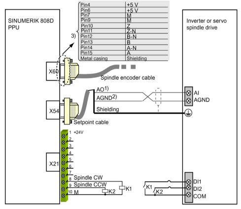
Figure 3-3 Connecting the inverter or the servo spindle drive (unipolar)
