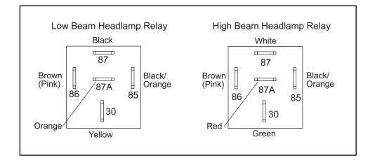
NOTE: Vehicles with DRL system require 8282 kit. Brown wires wiill be replaced by pink wires.
