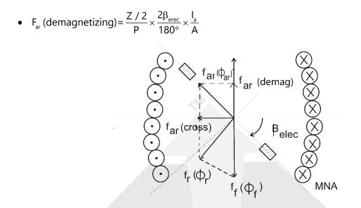
• Brush shift has serious limitations. Since, shift in MNA is proportional to Armature Current the brush has to be shifted in a new position every time the load changes, direction of rotation changes or mode of operation changes.
