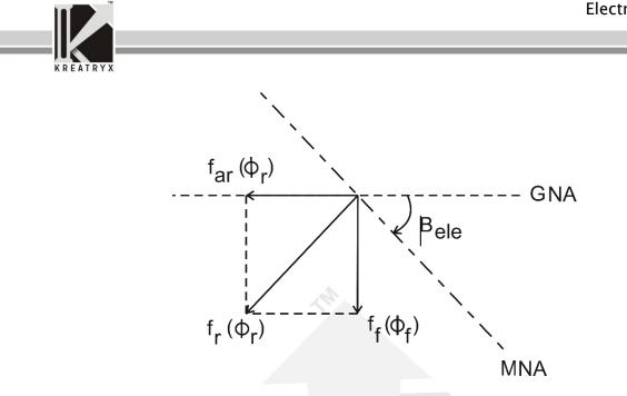
• Consequently, the MNA is no longer on the GNA but shifts in the direction of rotation for generator action and in a direction opposite to rotation for motor action.
