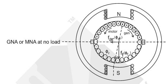
• Geometric Neutral Axis (GNA) is defined as the axis that is perpendicular to the field axis of the stator. Magnetic Neutral Axis (MNA) is defined as the axis perpendicular to the net flux that is flux due to field as well as armature mmf. The perpendicularity is taken in terms of electrical angle and not mechanical angle.
