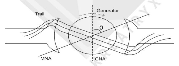
• If strengthening effect = weakening effect, the average flux under the pole remains same and therefore no demagnetizing effect of Armature Reaction. But due to saturation, strengthening effect < weakening effect so average flux under each pole reduces and hence Armature Reaction is demagnetizing.
