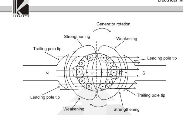
• Flux is strengthened where armature and field flux lie along the same direction and weakened where armature and field flux lie in opposite directions.
