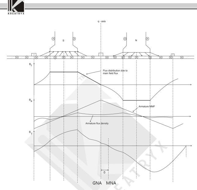
• Armature MMF from the above figure is triangular in shape and due to large air gap along q-axis the armature flux density is reduced along q-axis.
