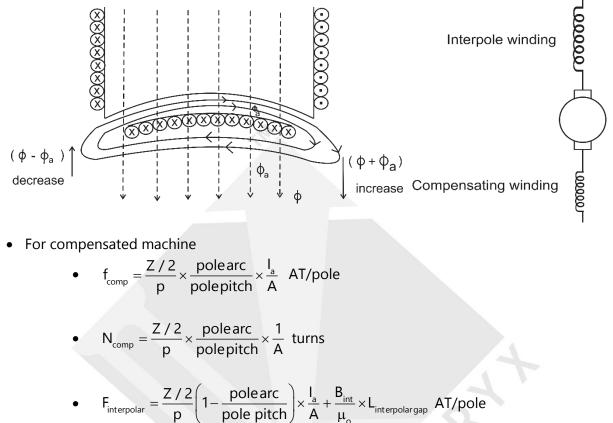
• Compensating winding reduces armature circuit inductance and therefore improves time response. Because it neutralizes AR under pole faces only.
