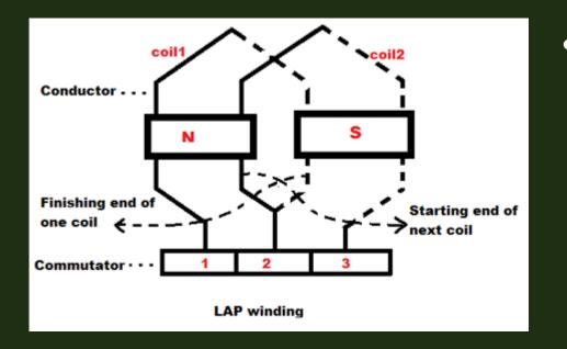
In this winding the finishing end of one coil is connected to one commutator segment and the starting end of the next coil situated under the same pole and connected with same commutator segment.
