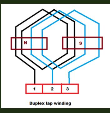
• A winding in which the number of parallel path between the brushes is twice the number of poles
