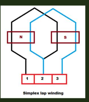
A winding in which the number of parallel path between the brushes is equal to the number of poles
