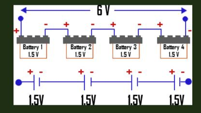
• The situation existing in a generator with regards to voltage and current is analogous to dry-cell connections.
