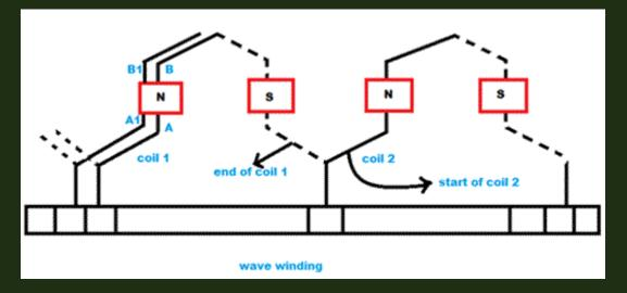
two ends of each coil are connected to commutator segments separated by the distance between poles
