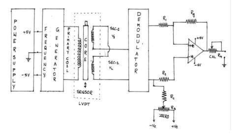
Fig – 13.1 Circuit Diagram of LVDT and Capacitance Pickup – Characteristics and Calibration
