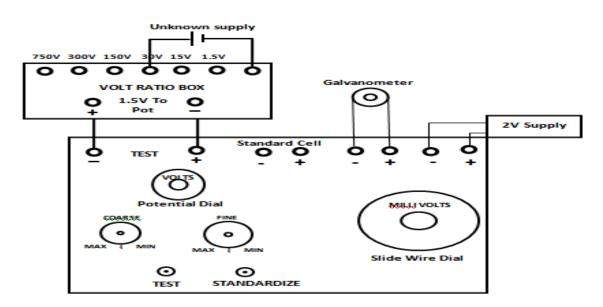
Fig – 3.2 Calibration of Voltmeter
