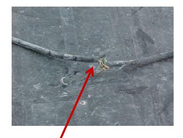
Damaged cord- remove from service
