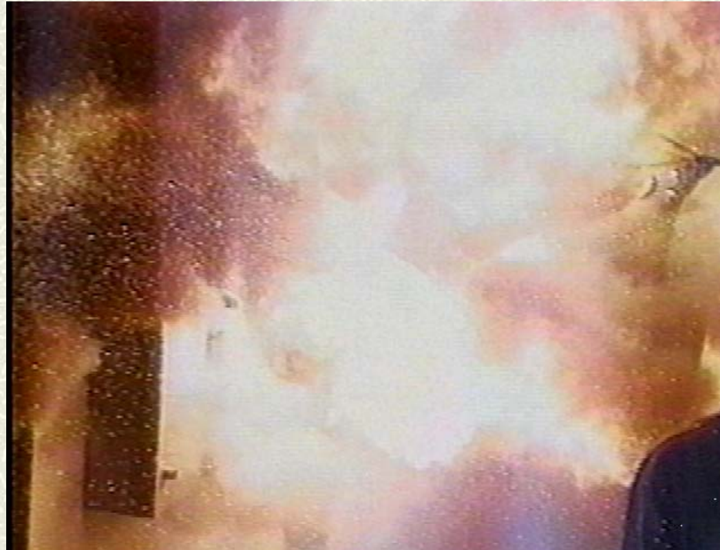
Example of an arcing fault
