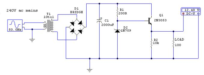
NOTE: This circuit above uses a 13 volt Zener diode, D2, which provides the voltage regulation. Approximately 0,6-0,7 volts are dropped across the transistor's b-e junction, leaving a higher current 12,3 volt output supply. This circuit can supply loads of up to 500 mA.
