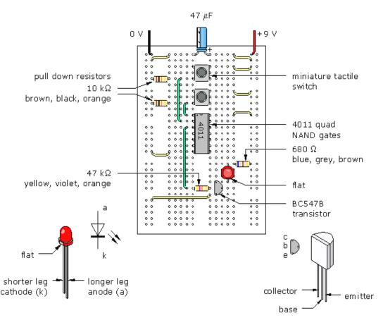
In the prototype circuit, it is not essential to make connections to the unused gates. However, in any final circuit, all unused CMOS inputs must be connected either to HIGH or to LOW. Make it an absolute rule that CMOS inputs are *never* left open circuit.
