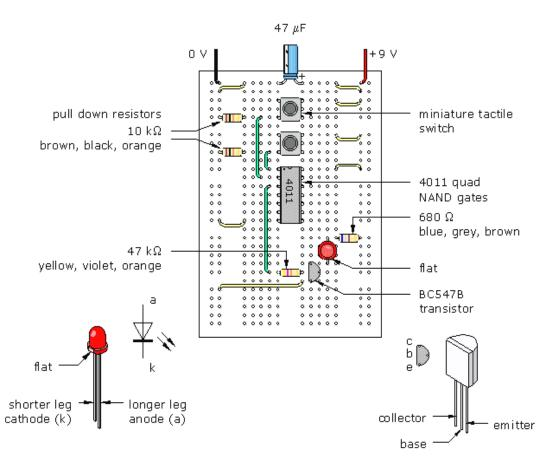
Proto-board Layout: The NAND gate test circuit
