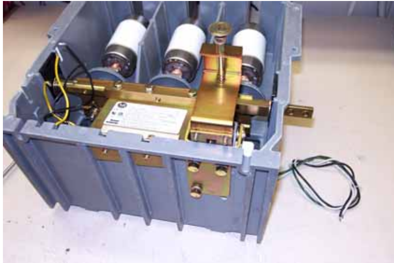
Figure 5 – Contactor (Front/bottom View) Showing Mounting Bolts for Latch Mechanism
