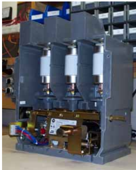
Figure 7 – Contactor (front angle view) after Auxiliary Actuator Plate is re-assembled
