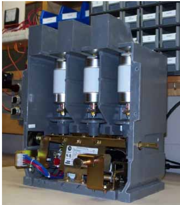
Figure 11 – Complete Contactor after Conversion
