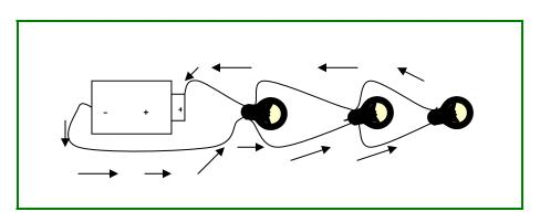
• Batteries in a series: are two or more batteries connected to make a circuit. The negative electrode of one battery is connected to the positive electrode of the next battery. Batteries in a series will increase the voltage (there will be more electricity flowing).
