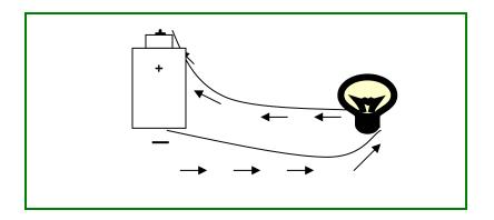
• A series circuit: When you have more than one device connected to a continuous circle of wire, for example two light bulbs. The electricity must travel through everything in the circuit before it returns to the battery. When one light goes out in a series circuit, the other lights go out too.
