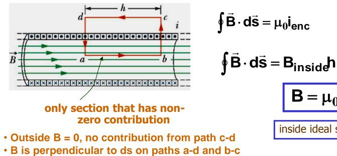
Inside B is uniform and parallel to ds on path a-b
